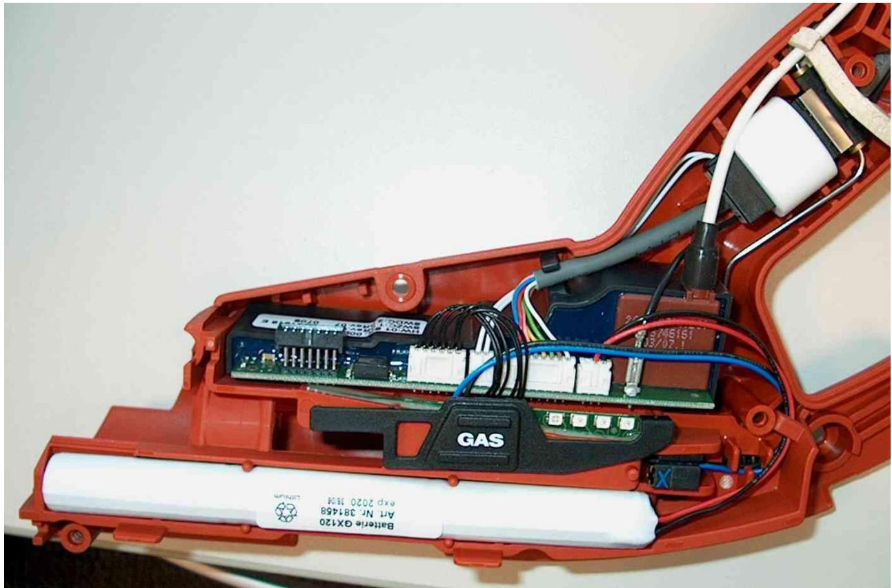
This picture shows the RFID reader PCB alone. In the left you will see the coil for the 125 kHz communication with the transponder:
