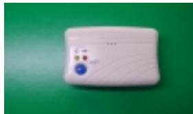
Switch on to check if yellow light is blinking (indicating batteries are correctly inserted). If the light is not blinking, repeat above procedure.
