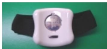
Insert new battery securely in place, with words facing up.
