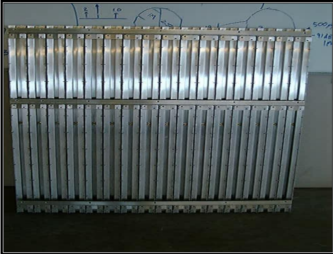
PHOTOGRAPH 10: BACK OF ANTENNA ARRAY
