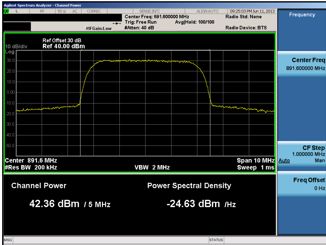
Plot 6-9. Maximum Conducted Power (High Ch – 891.6MHz – 64QAM)
