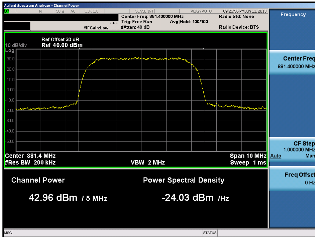
Plot 6-5. Maximum Conducted Power (Mid Ch – 881.4MHz – 16QAM)
