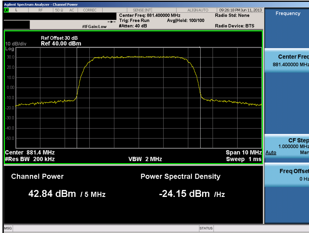
Plot 6-4. Maximum Conducted Power (Mid Ch – 881.4MHz - QPSK)
