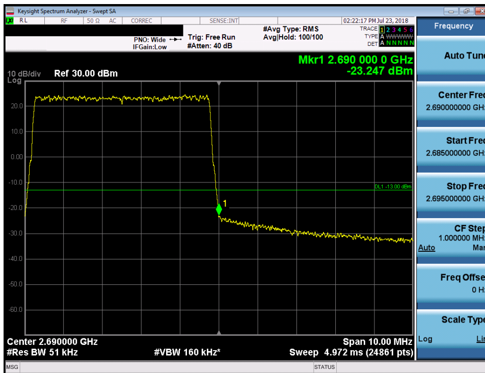
Plot 7-225. Upper Band Edge Plot (Band 7 - 5.0MHz 256-QAM)
