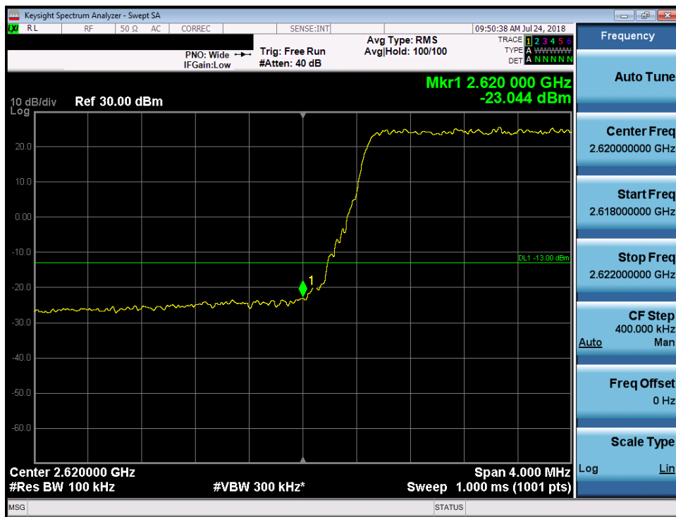
Plot 7-235. Lower Band Edge Plot (Band 7 - 10.0MHz 64-QAM)
