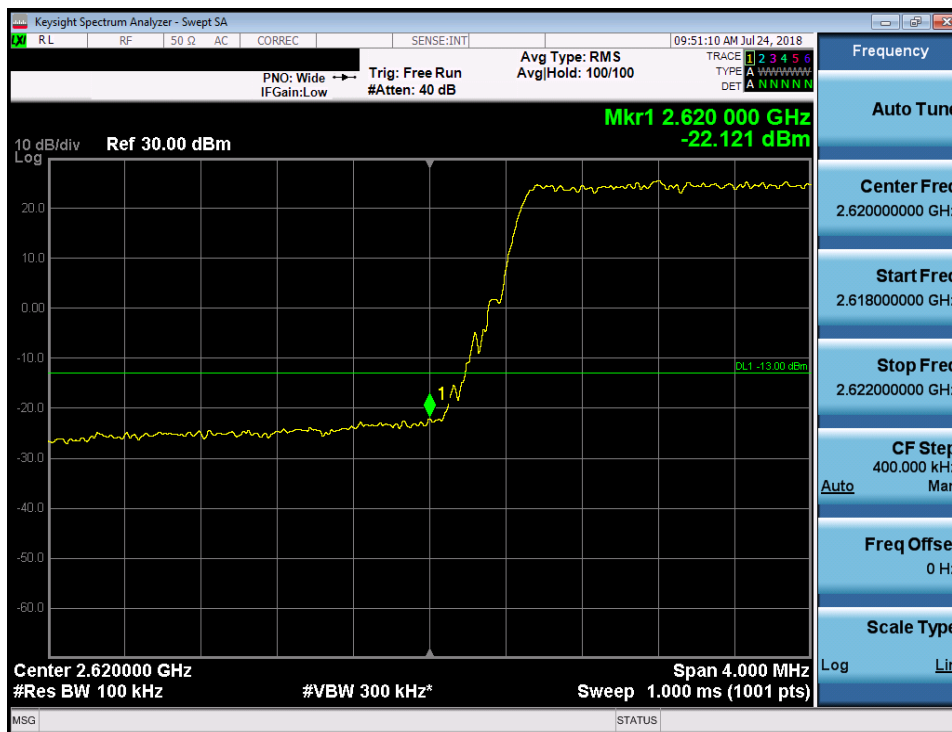
Plot 7-239. Lower Band Edge Plot (Band 7 - 10.0MHz 256-QAM)
