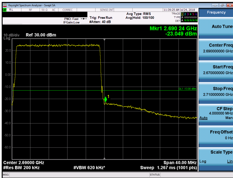
Plot 7-269. Upper Band Edge Plot (Band 7 - 20.0MHz 64-QAM)
