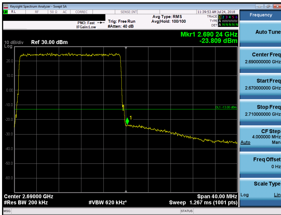
Plot 7-273. Upper Band Edge Plot (Band 7 - 20.0MHz 256-QAM)
