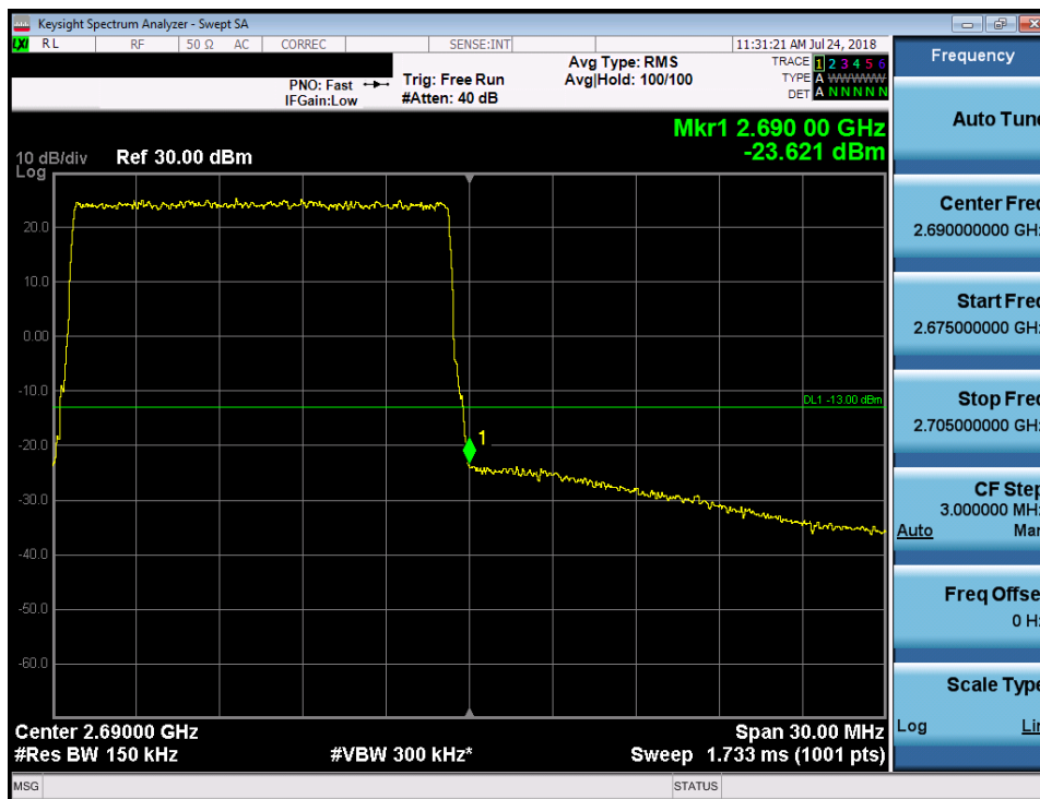
Plot 7-245. Upper Band Edge Plot (Band 7 - 15.0MHz QPSK)
