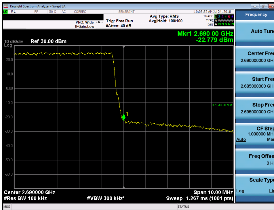
Plot 7-233. Upper Band Edge Plot (Band 7 - 10.0MHz 16-QAM)
