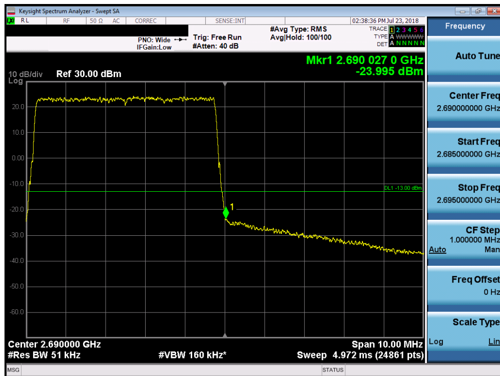
Plot 7-157. Upper Band Edge Plot (Band 7 - 5.0MHz 64-QAM)
