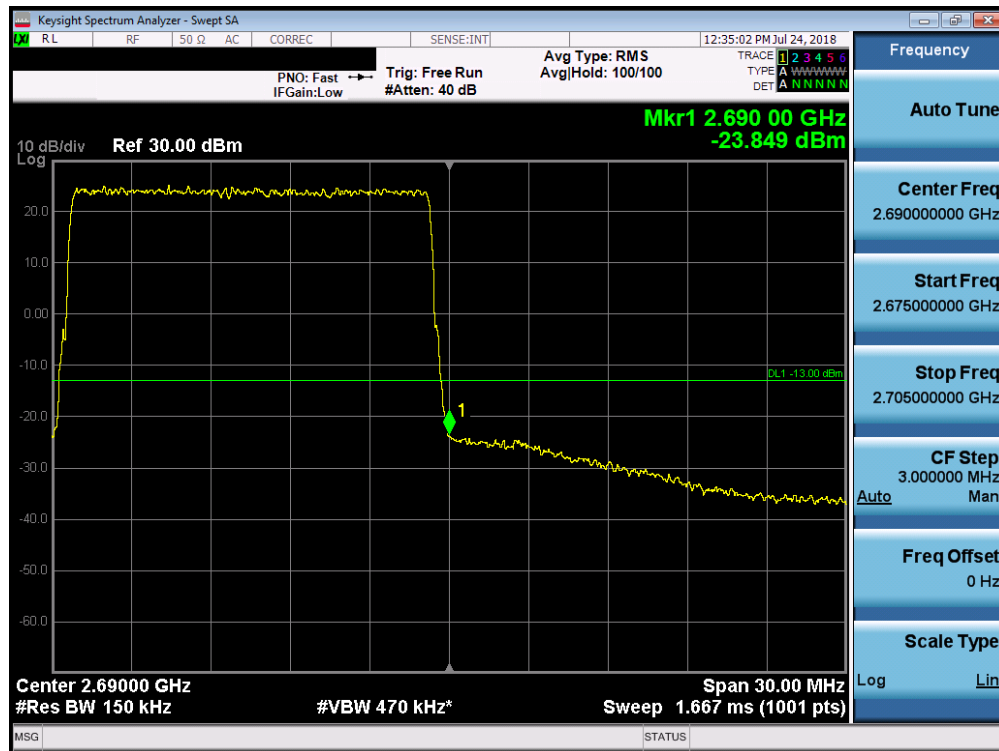
Plot 7-189. Upper Band Edge Plot (Band 7 - 15.0MHz 64-QAM)
