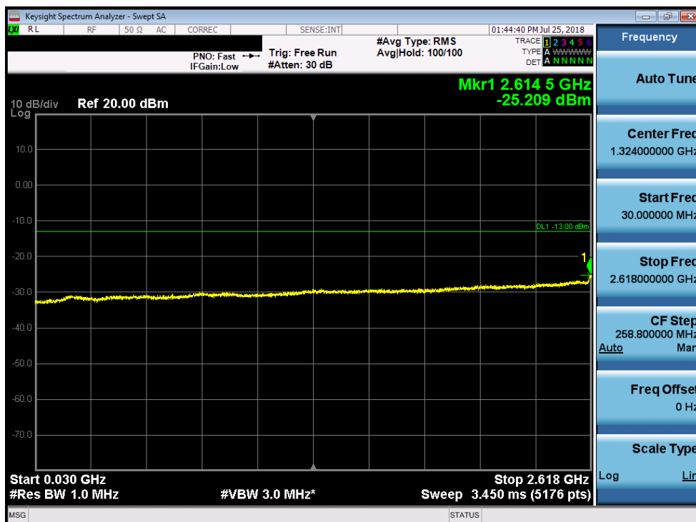
Plot 7-132. Conducted Spurious Plot (Band 7 - 10.0MHz QPSK – Mid Channel)
