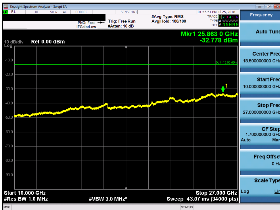
Plot 7-134. Conducted Spurious Plot (Band 7 - 10.0MHz QPSK – Mid Channel)
