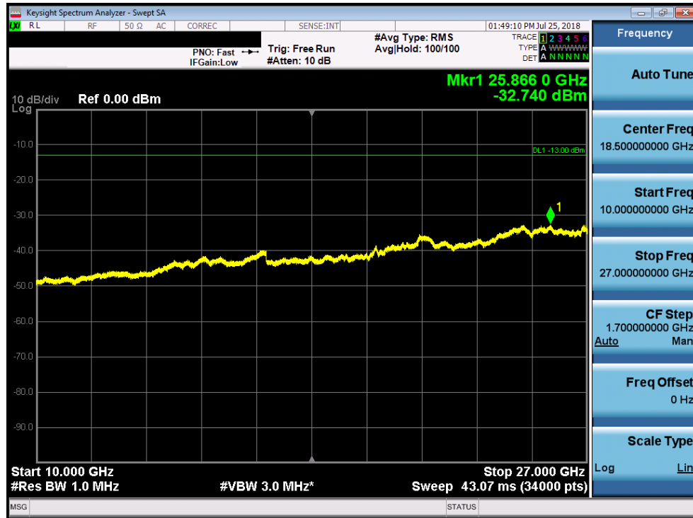
Plot 7-137. Conducted Spurious Plot (Band 7 - 10.0MHz QPSK – High Channel)
