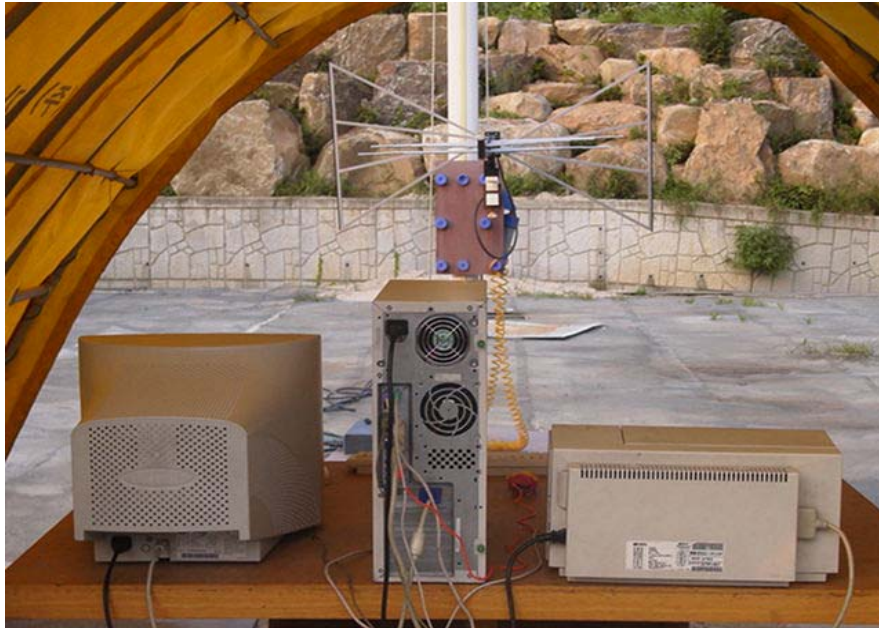
Photograph 1 : Setup for radiated Emissions
