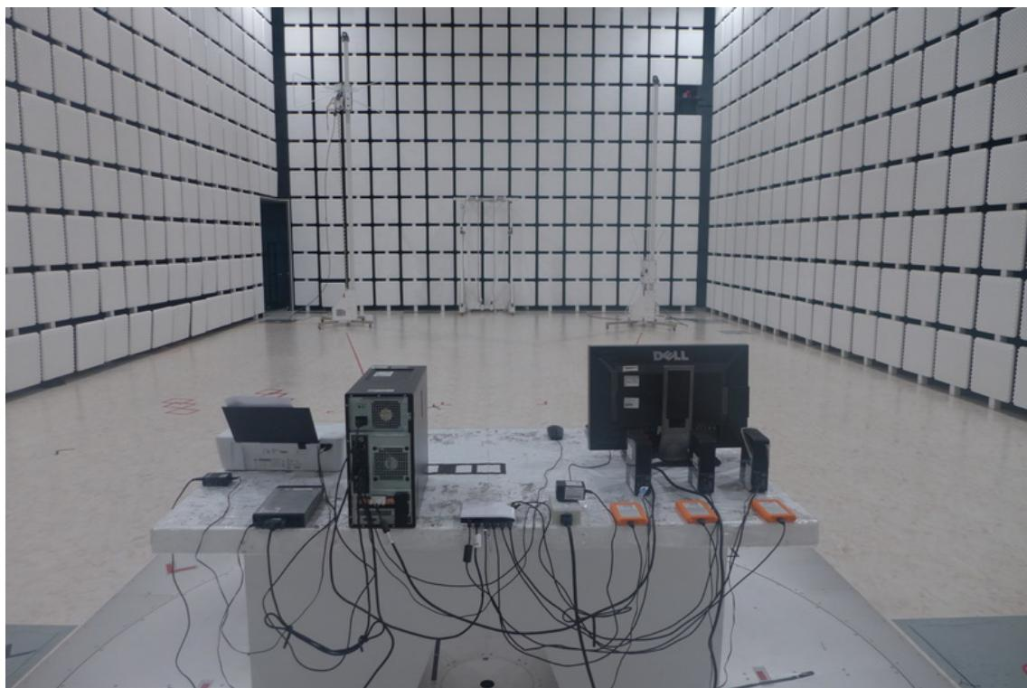
**Radiated emission test photos**
