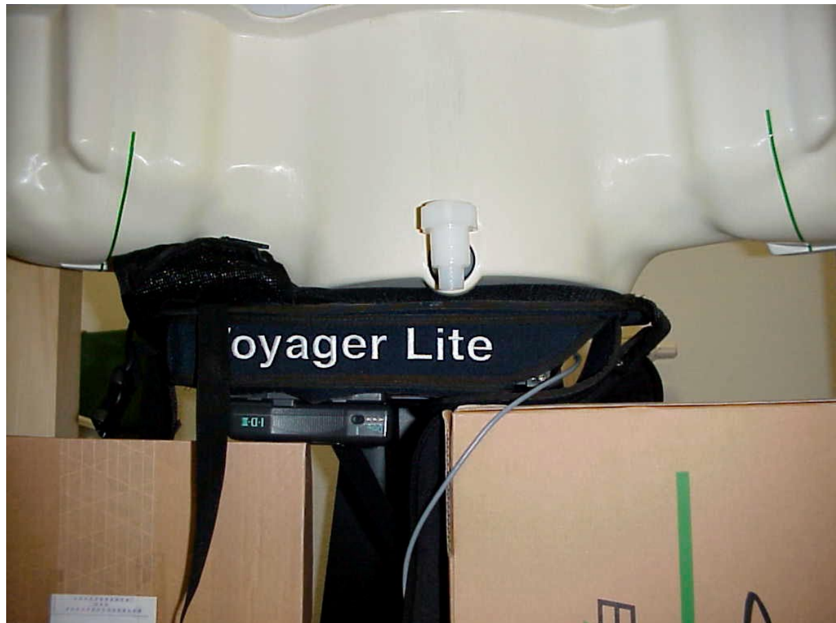
Photo 5: Body measurement (flat phantom) transmitter with rucksack
