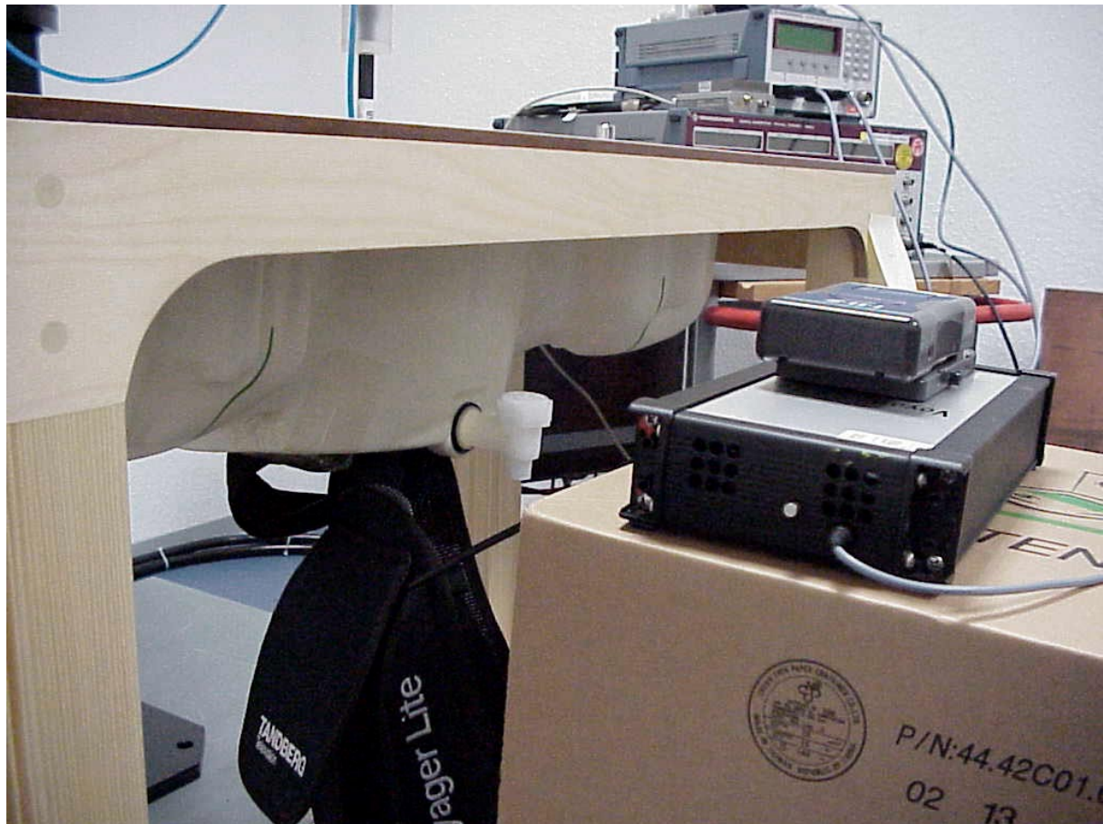
Photo 2: Patch antennas against the body phantom
