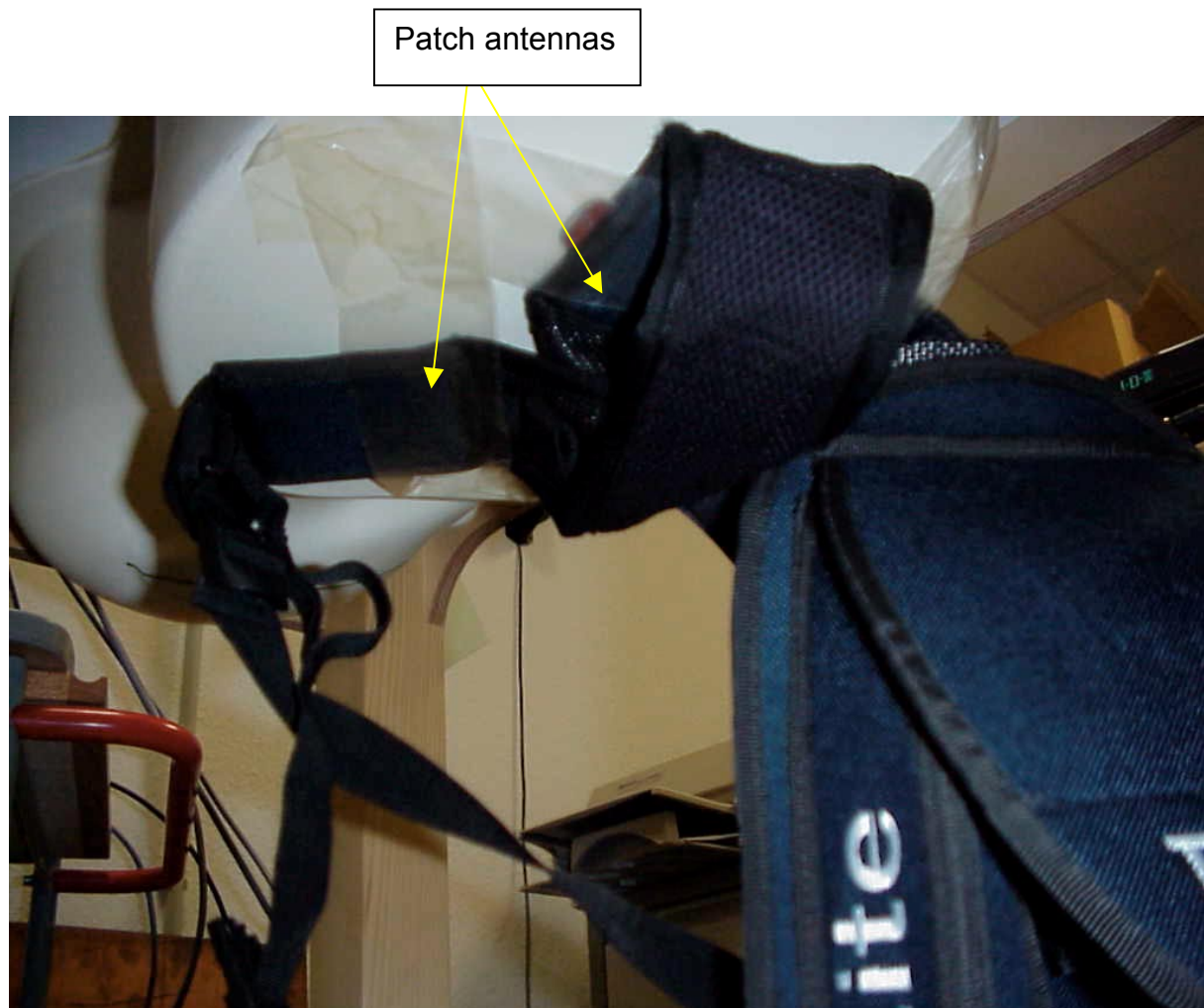
Photo 3: Patch antennas against the body phantom under view
