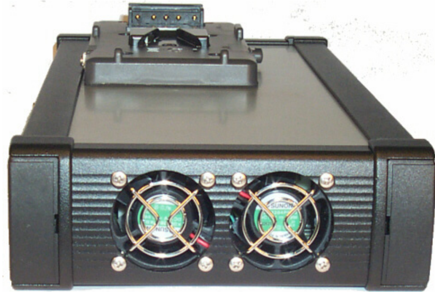
Figure 1.5: View Showing Exhaust Fans in Top Panel
