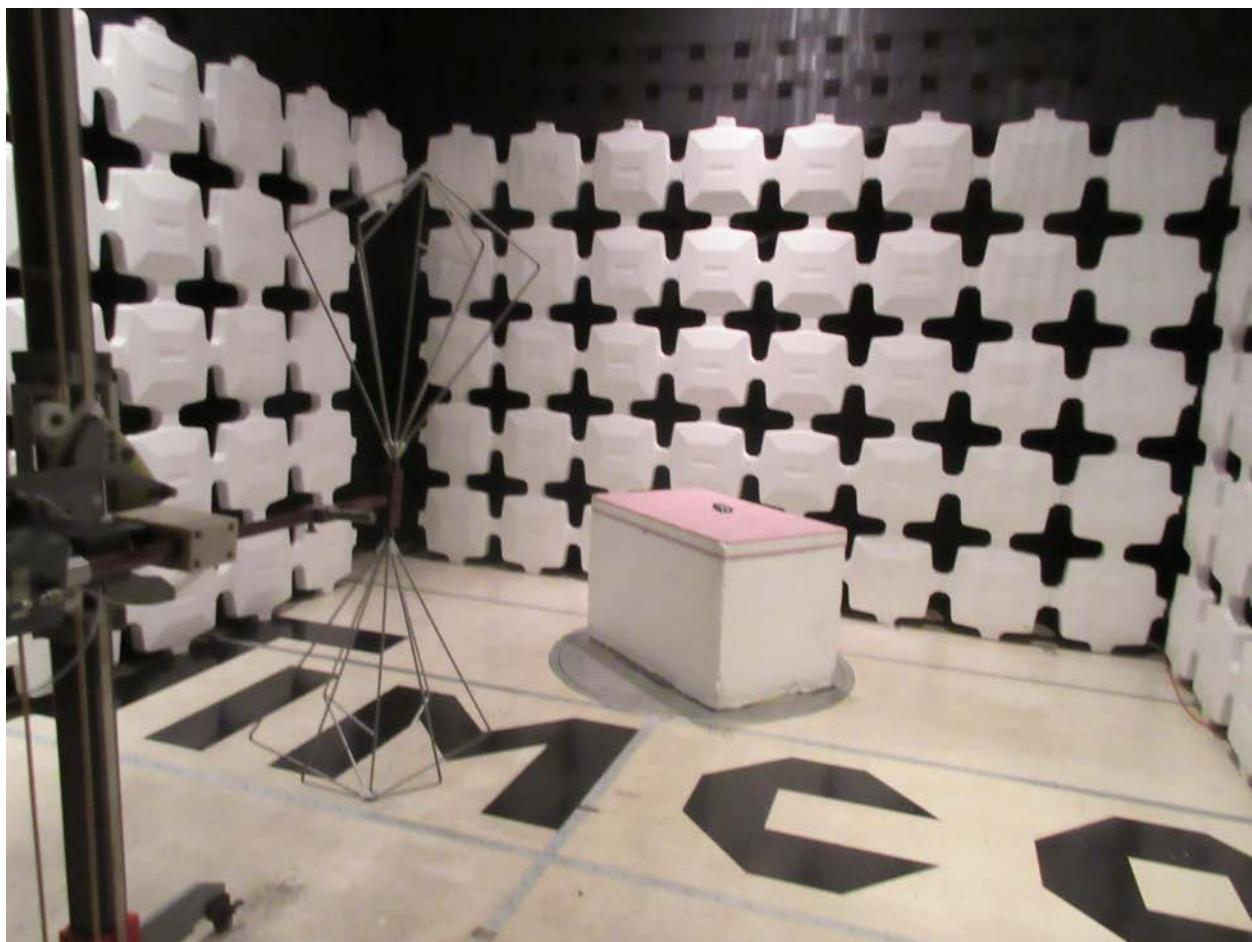
**Radiated Tests Above 1 GHz: In Band Field Strength/Restricted Band Emissions**
