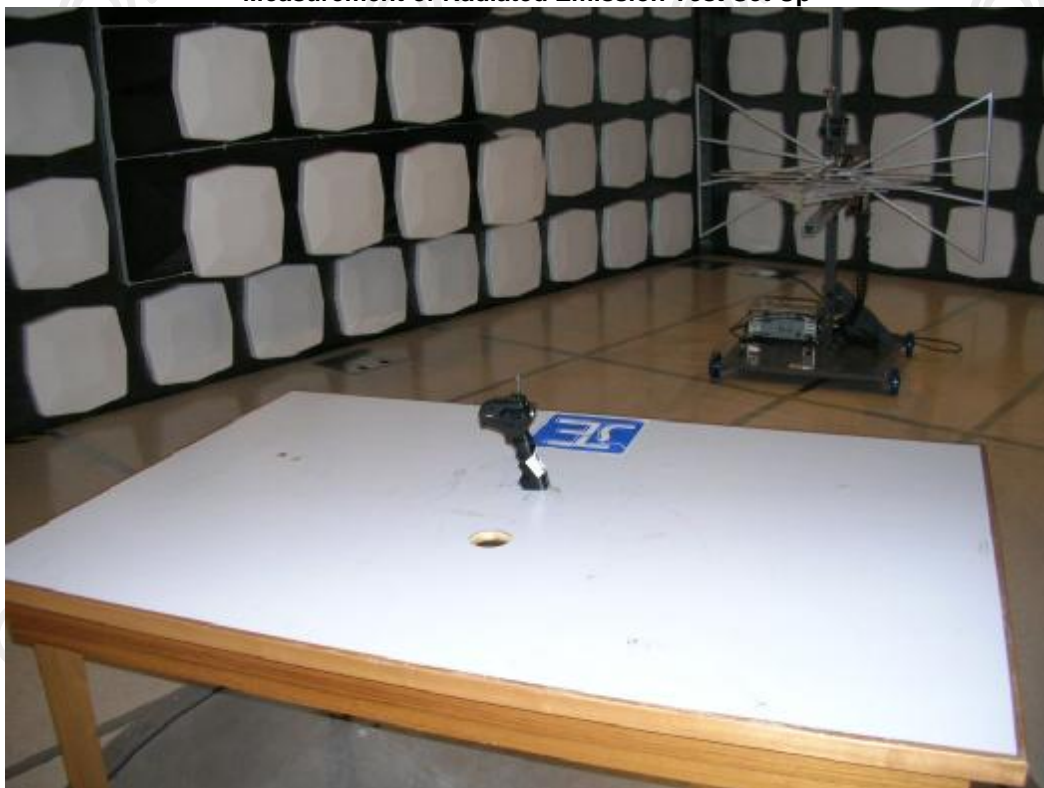
Measurement of Radiated Emission Test Set Up
