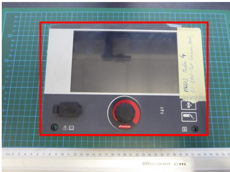
During normal operation the EUT can be paired with an ancillary Smartphone/Laptop to configure the welding parameters via remote control.
