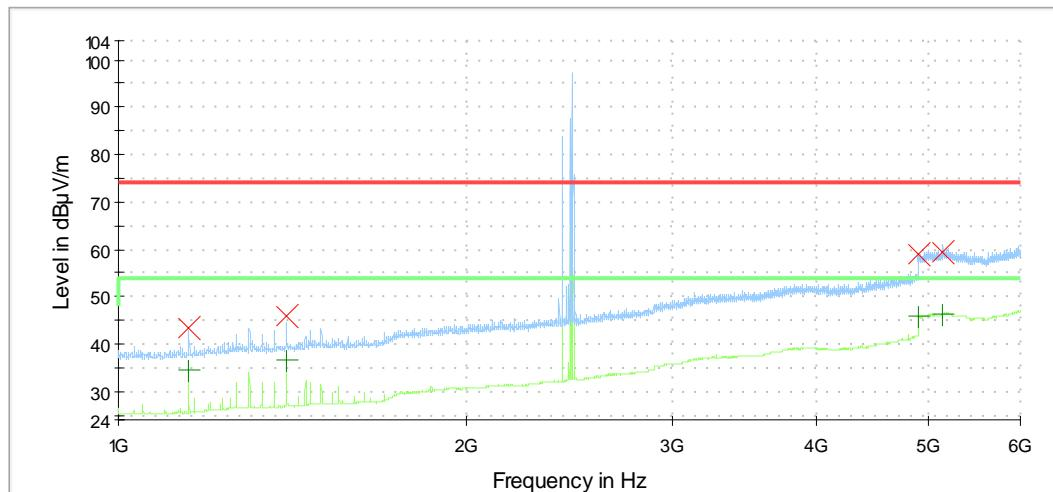
The results of the standard subsequent measurement above 1 GHz in an anechoic chamber are indicated in the table below. The limits as well as the measured results (levels) refer to the above mentioned standard while taking account of the specified requirements for a 3 m measuring distance.
