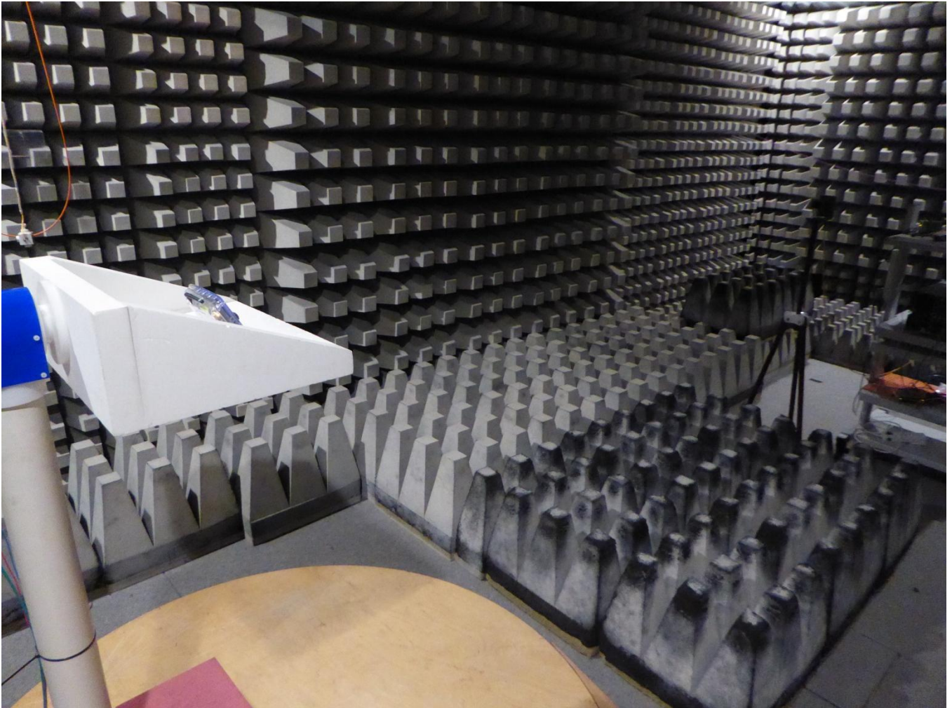
Test setup fully anechoic chamber Preliminary & final measurement 18 – 26.5 GHz
