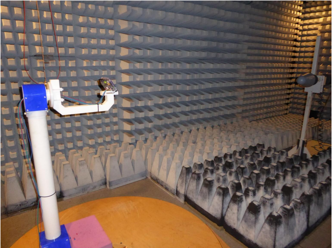
Test setup fully anechoic chamber Preliminary & final measurement 1 – 12 GHz
