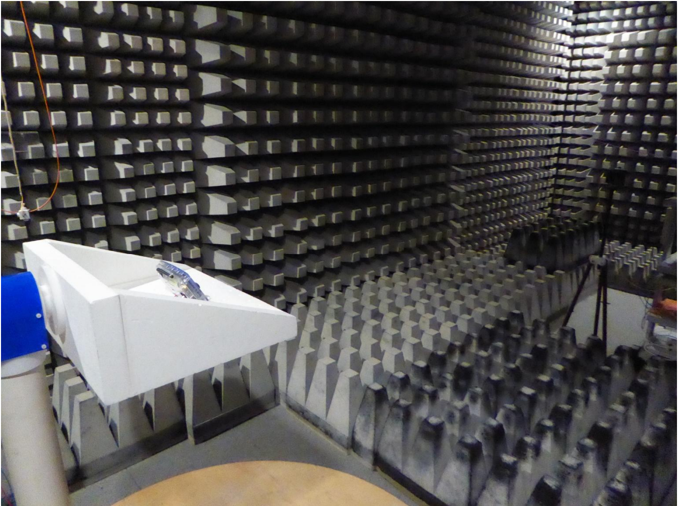
Test setup fully anechoic chamber Preliminary & final measurement 12 - 18 GHz
