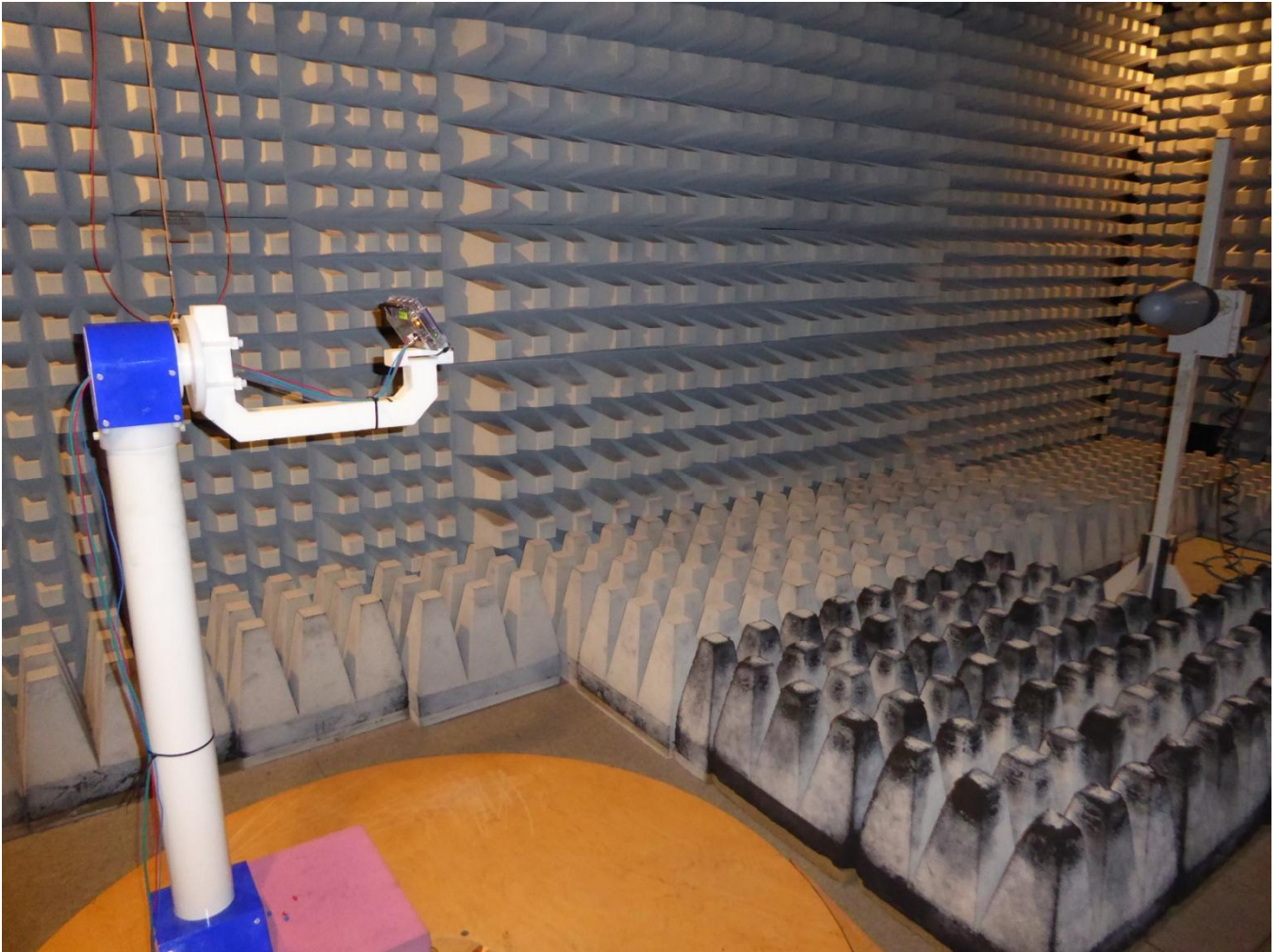
Test setup fully anechoic chamber Preliminary & final measurement 1 – 12.75 GHz
