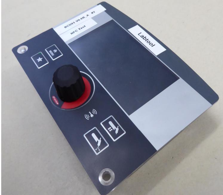
During normal operation the EUT can be paired with an ancillary Smartphone/Laptop to configure the welding parameters via remote control.
