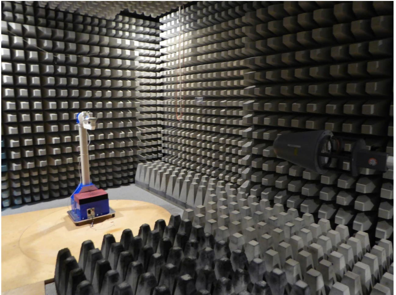
Test setup fully anechoic chamber Preliminary and final measurement 1 – 12 GHz
