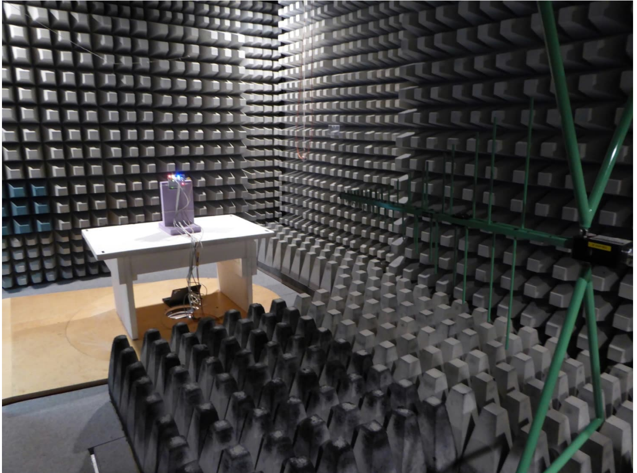
Test setup fully anechoic chamber Preliminary measurement 30 MHz – 1 GHz
