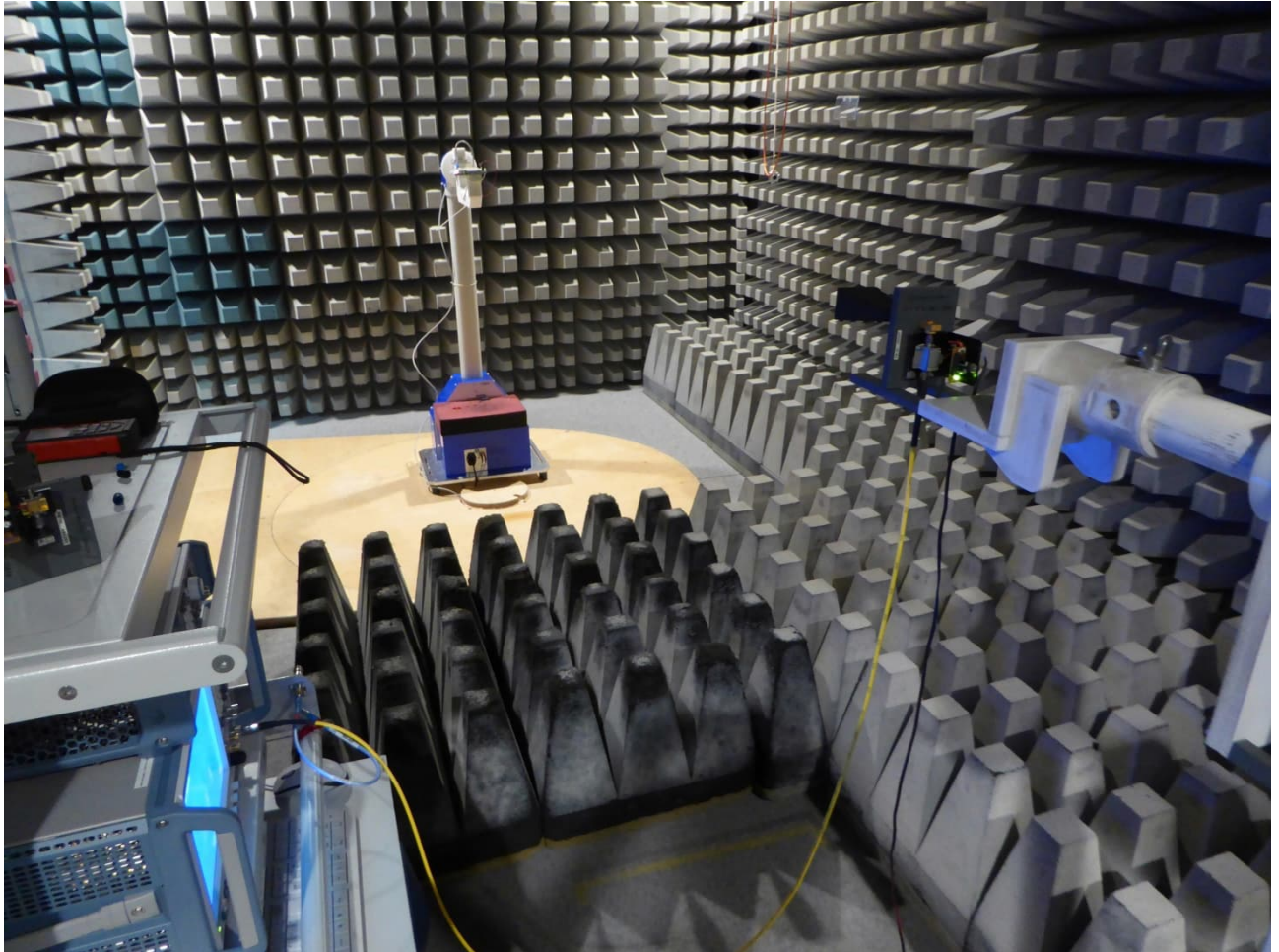
Test setup fully anechoic chamber Preliminary and final measurement 18 –26.5 GHz
