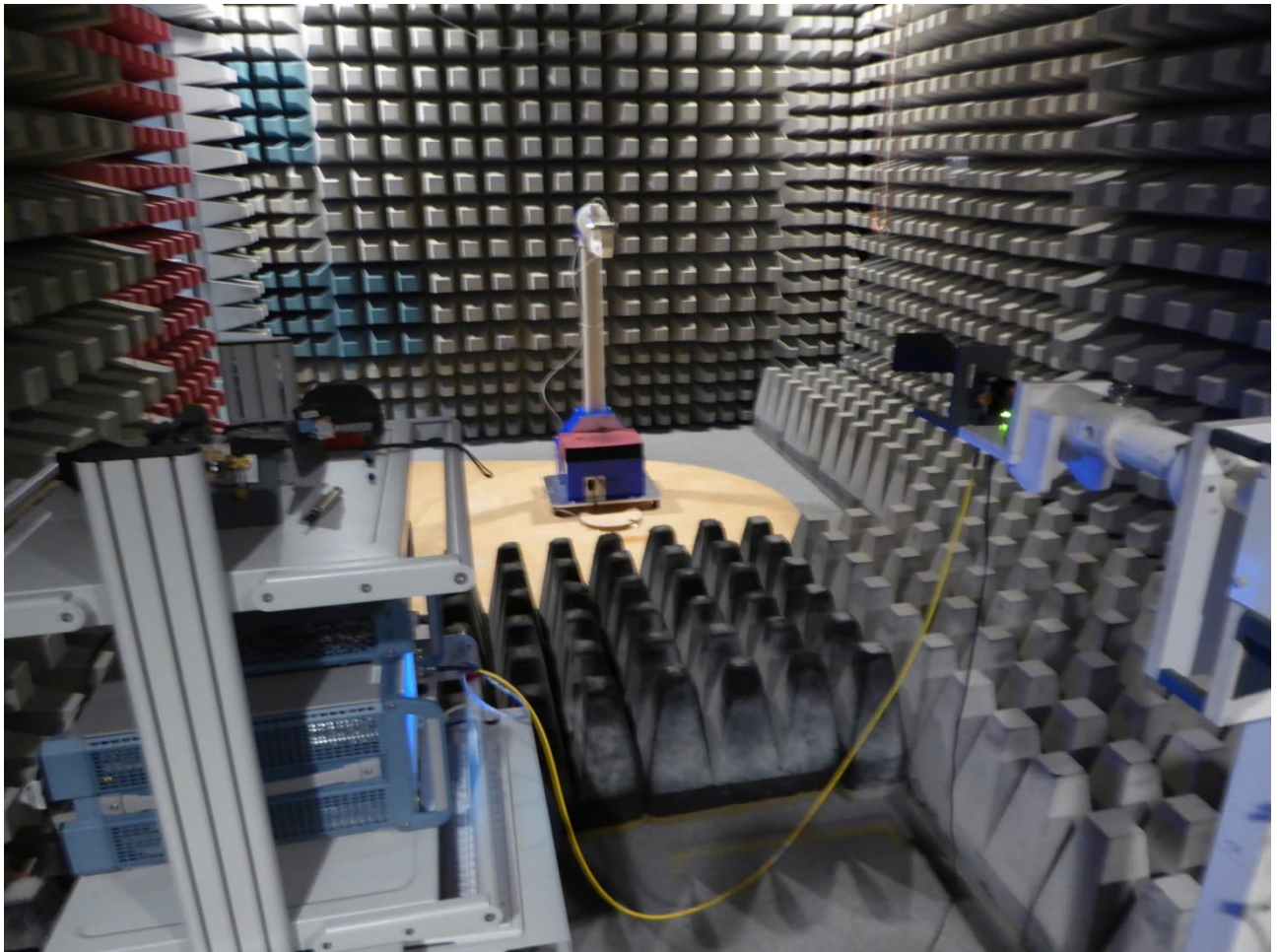
Test setup fully anechoic chamber Preliminary and final measurement 12 –18 GHz
