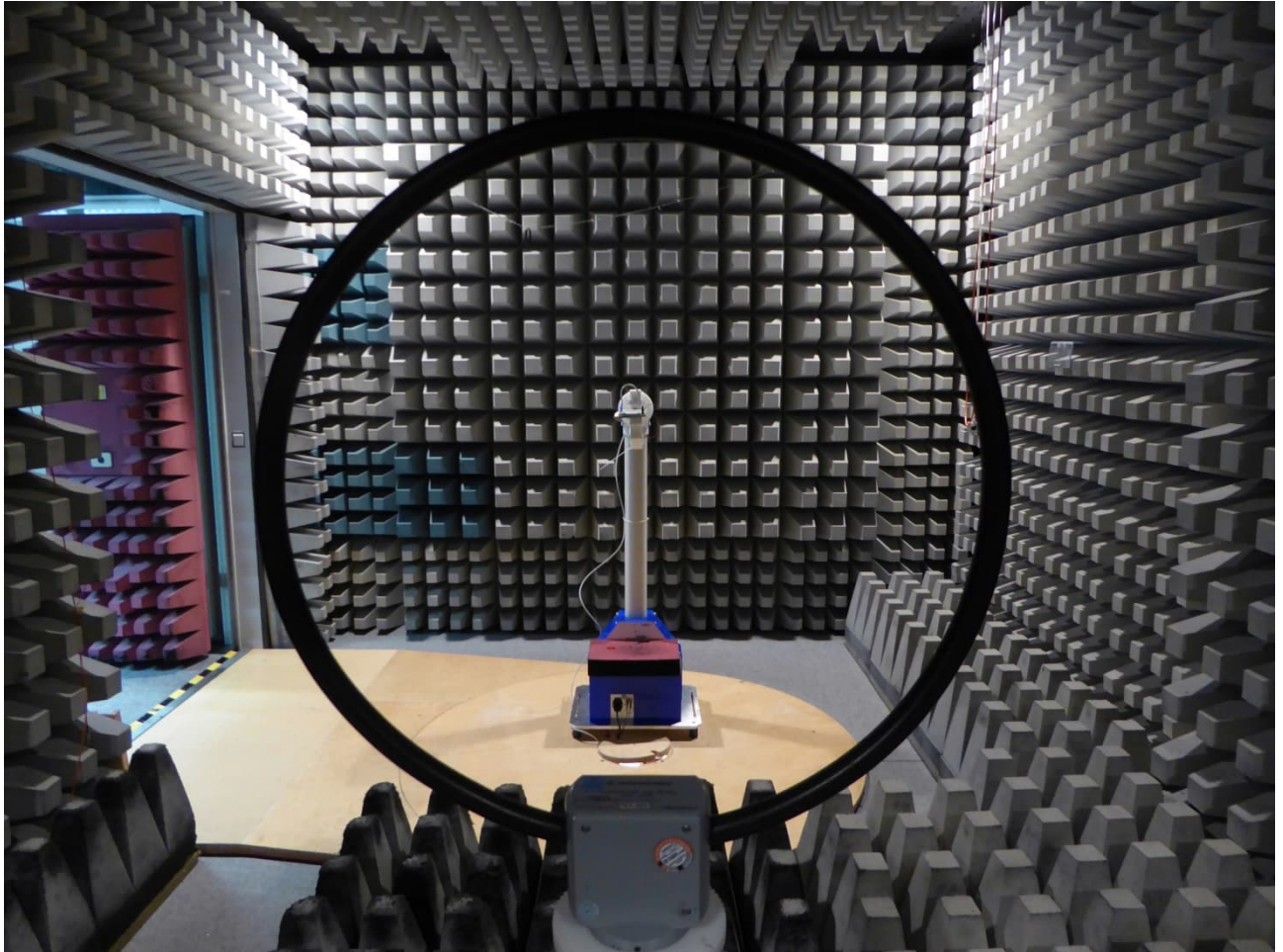
Test setup fully anechoic chamber Preliminary measurement 9 kHz – 30 MHz
