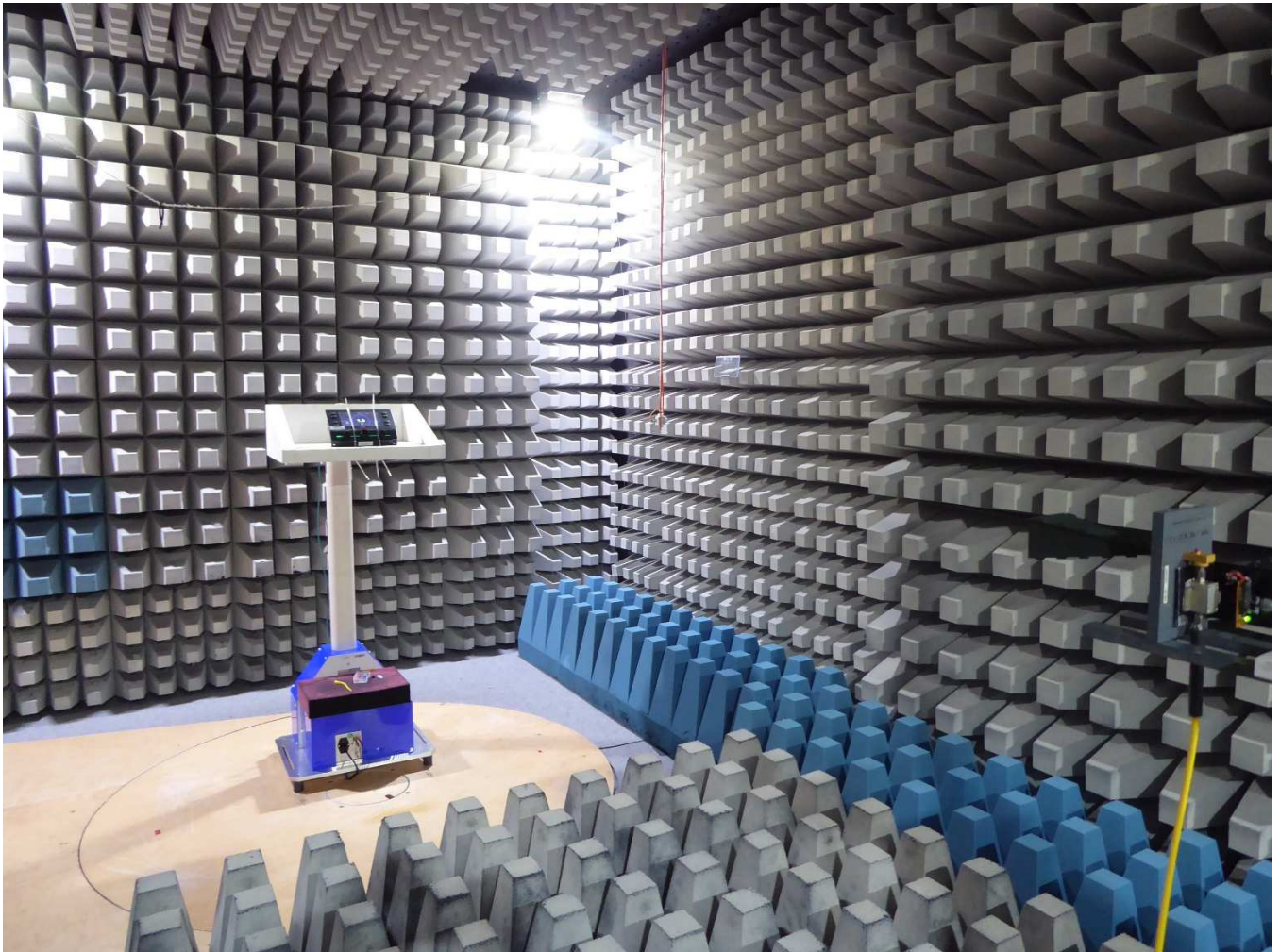
Test setup fully anechoic chamber TX 18 GHz – 26.5 GHz
