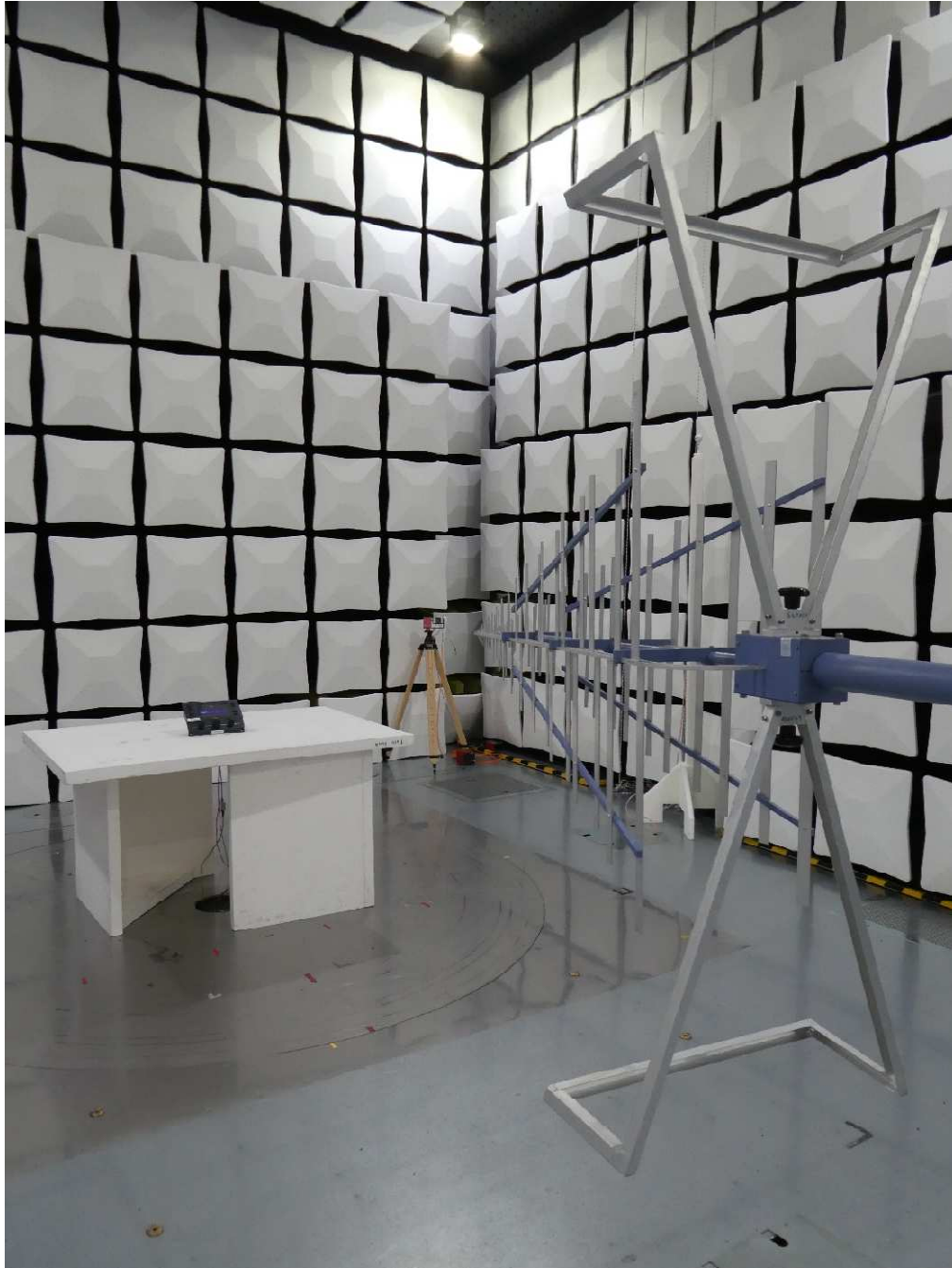
Test setup semi anechoic chamber TX 30 MHz – 1 GHz
