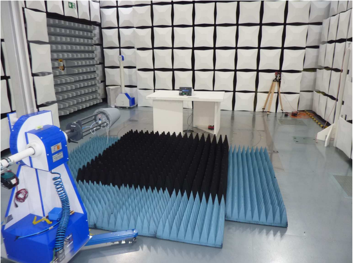
Test setup semi anechoic chamber 1 – 13 GHz
