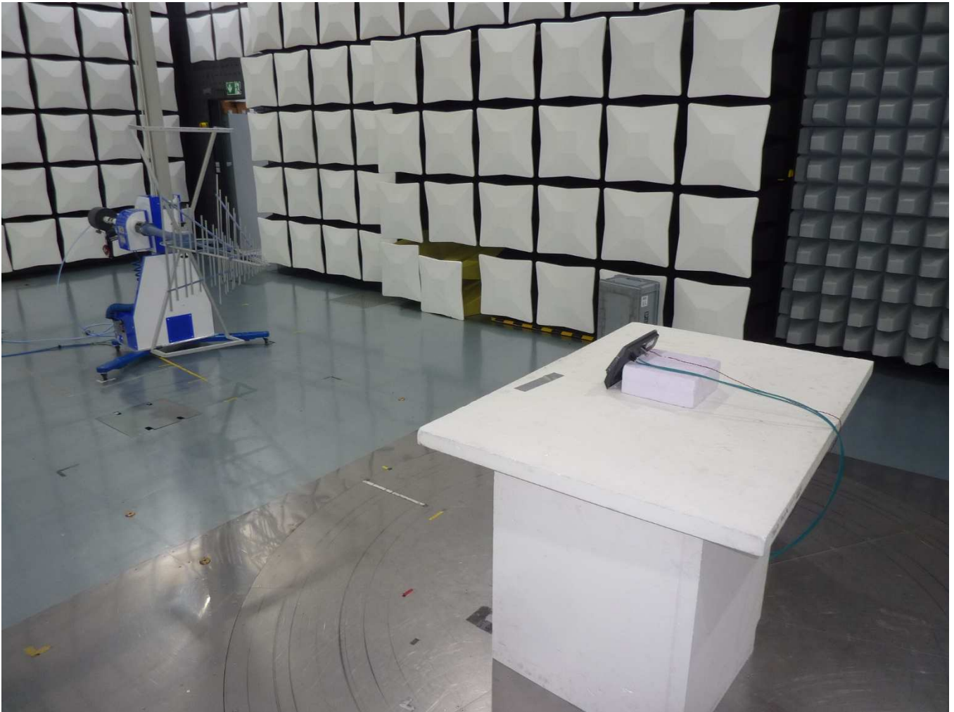
Test setup semi anechoic chamber 30 – 1000 MHz
