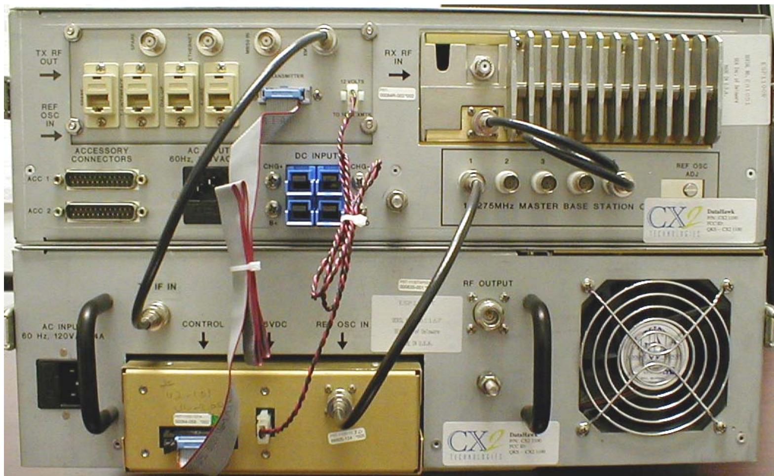
Figure 5.2 External Back View (showing interconnections)
