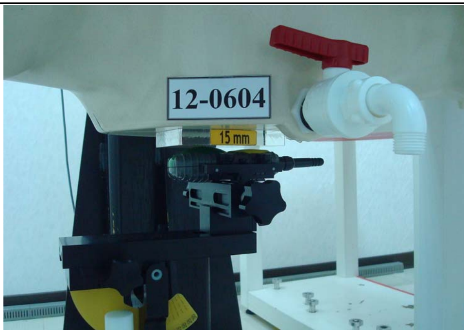
Figure 2. Brain SAR Test Setup (Flat Section)
