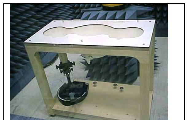
Figure 5. SAM Twin Phantom
