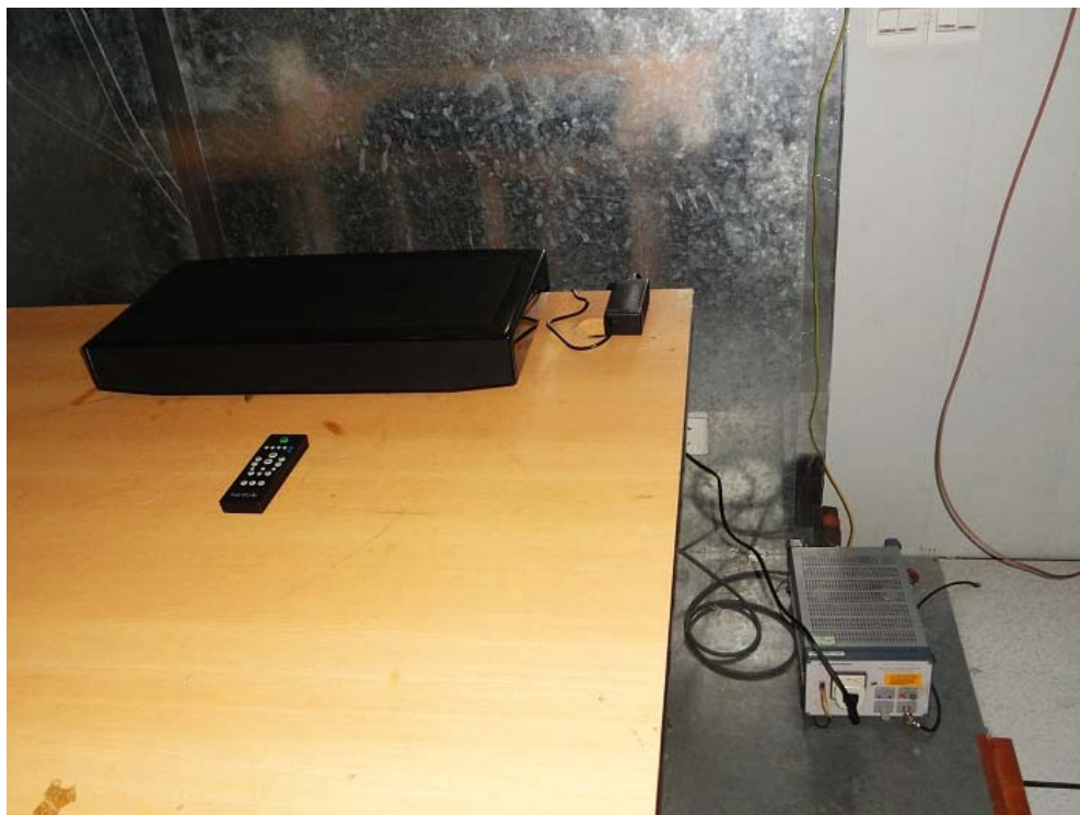
Conducted Emission Test Setup:
