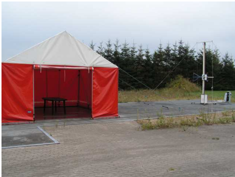
TXFH-RC field strength measurement below 1GHz and at 10m distance
