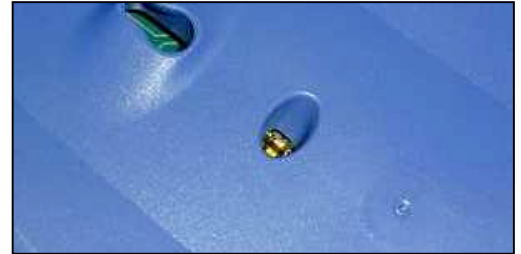
Figure 1 . Factory settings switch is located on the back of Ailonet.
