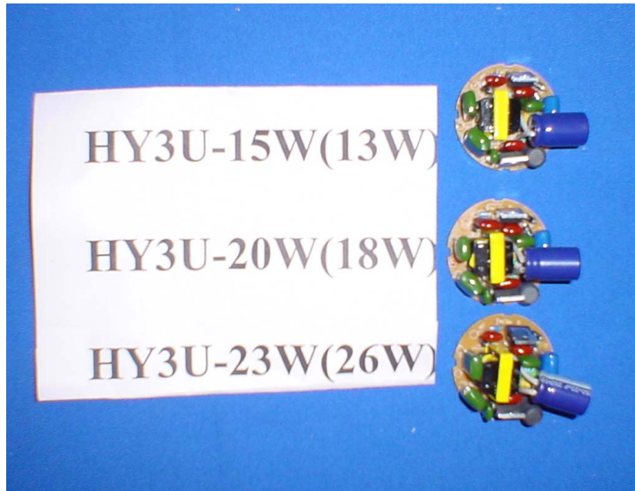
Figure 3 M/N: HY3U Series Main Board, Component Side
