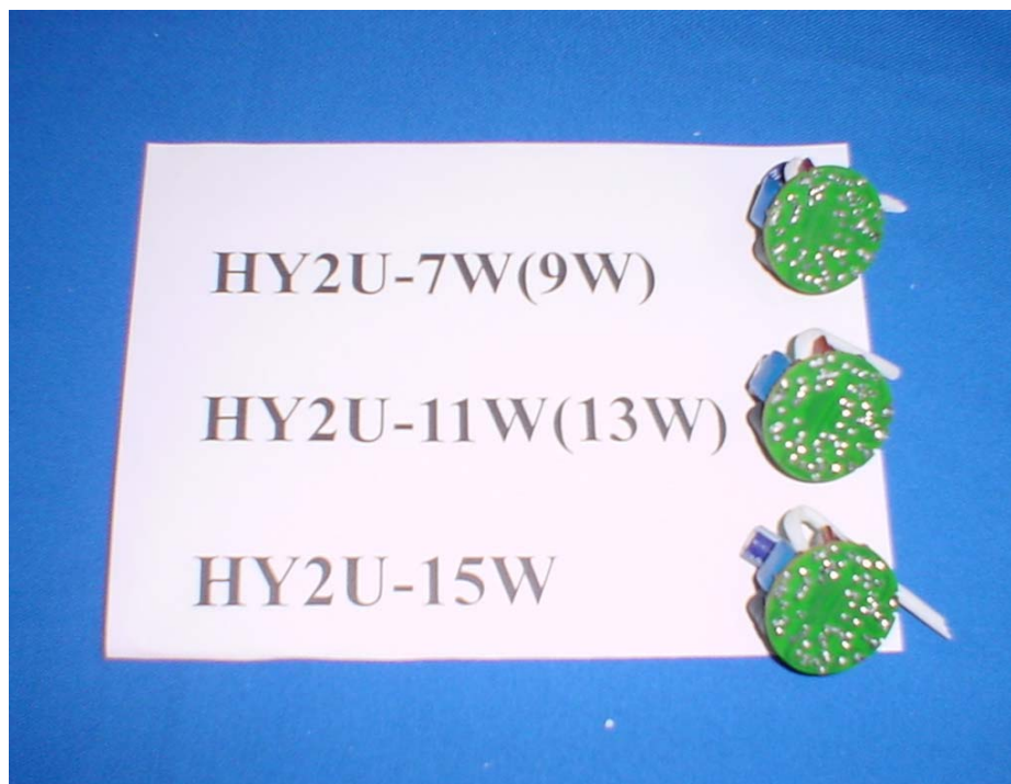
Figure 2 M/N:HY2U Series Main Board, Soldered Side
