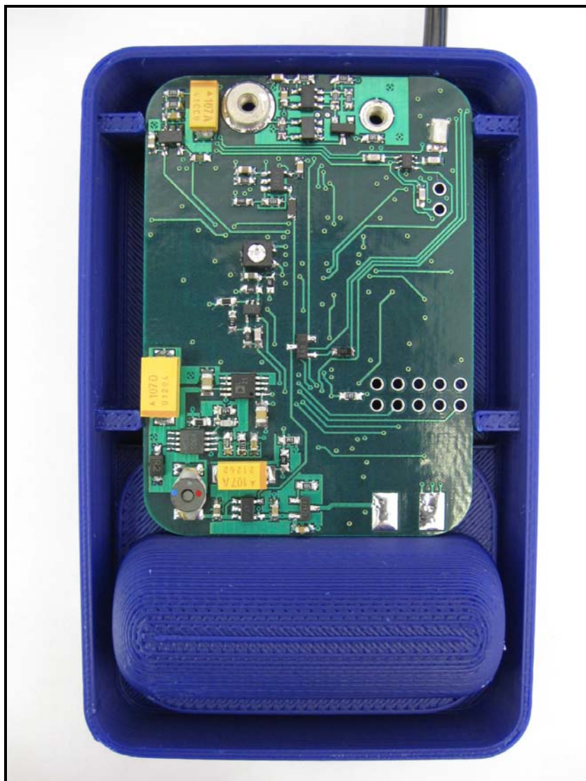
Photograph 5: PCB in Enclosure
