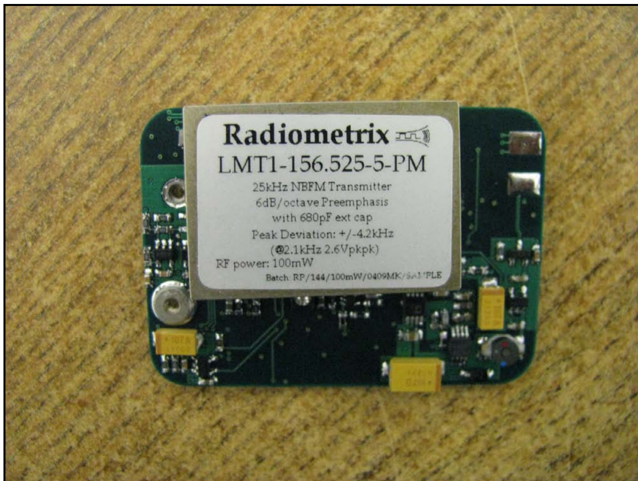
Photograph 8: Main PCB – Top with DSC Transmitter
