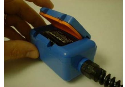
Figure 4. CORRECT gasket seating
