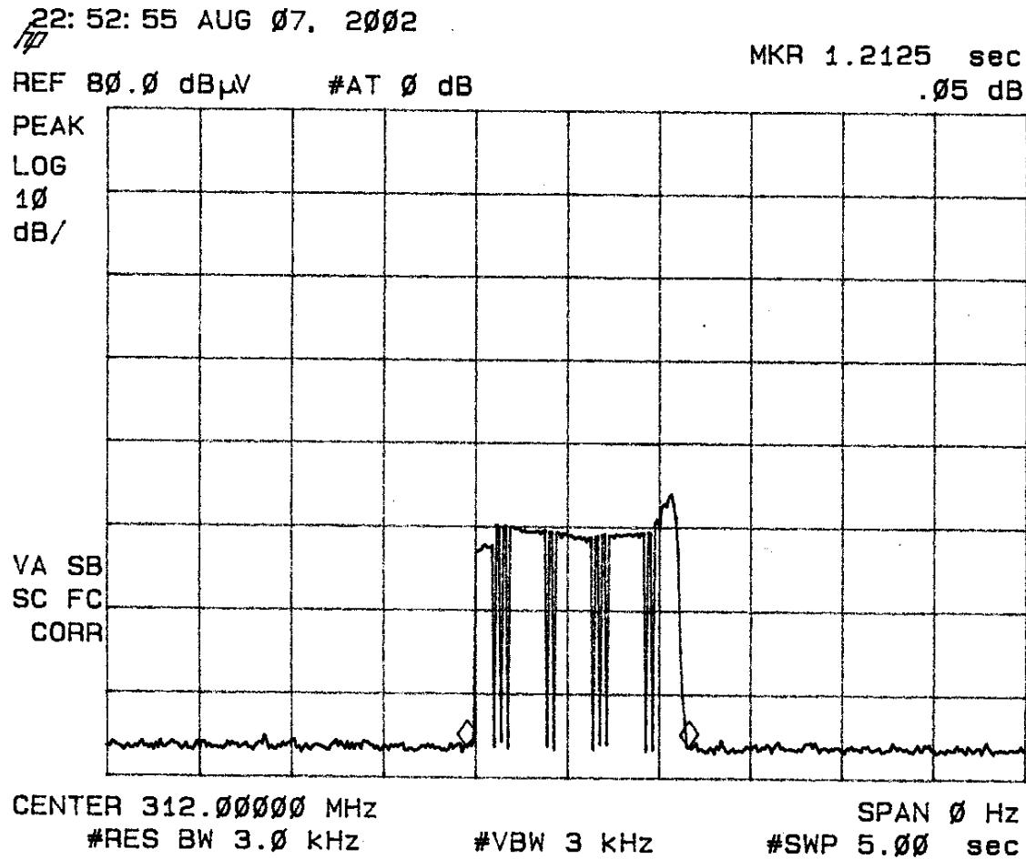
『**Remark:** The device (Wireless Door Bell Remote Control/Transmitter, EUT) is a manually operated transmitter, that is automatically deactivated the transmitter within not more than 5 seconds of being released. Compliance with §15.231 (a)- (1).』
