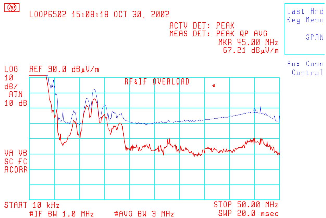
**Plot #3(b) - Upper 10 dB BW Point of the TLF with 50 MHz Antenna
