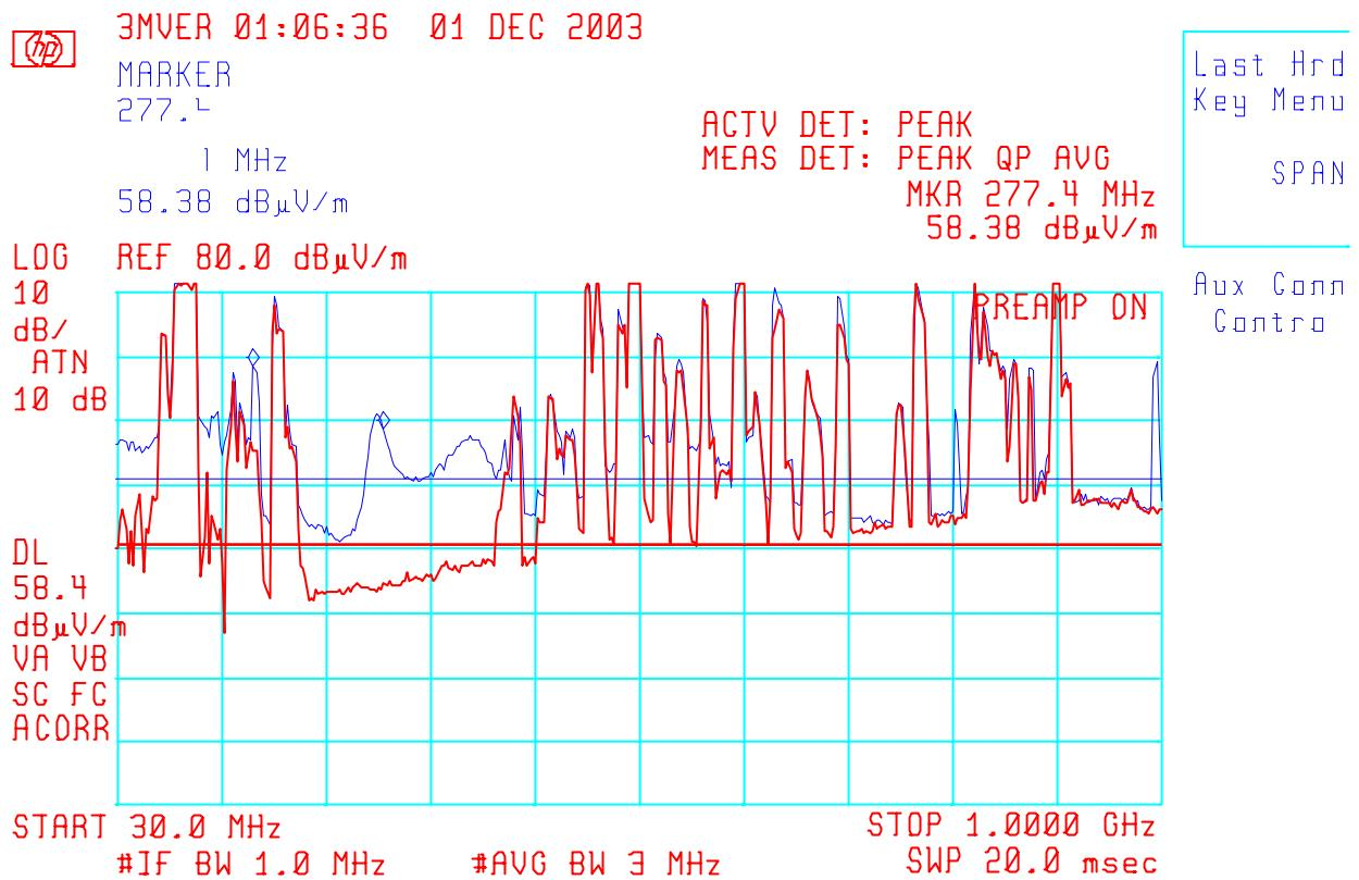
Plot #3(a) - Lower 10 dB BW Point of the TLF with 50 MHz Antenna
