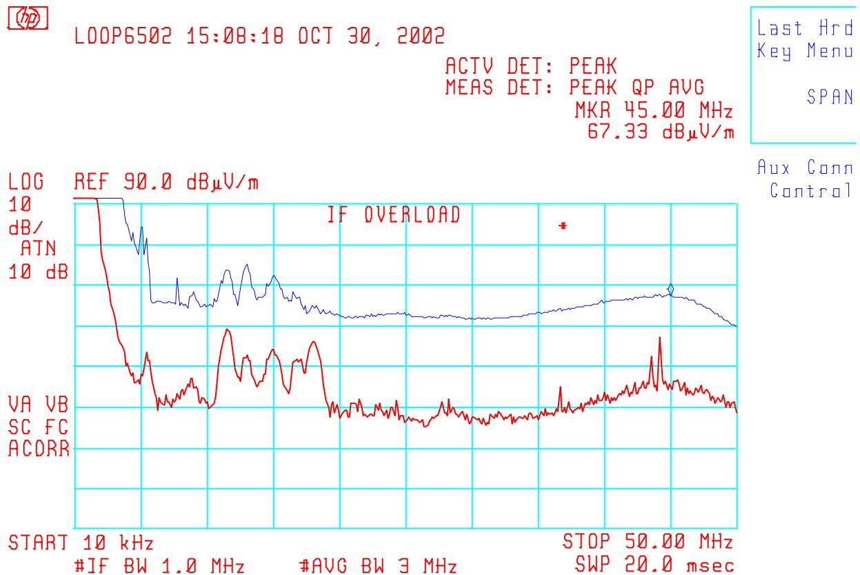
**Plot #2(b) - Upper 10 dB BW Point of the TLF with 100 MHz Antenna
