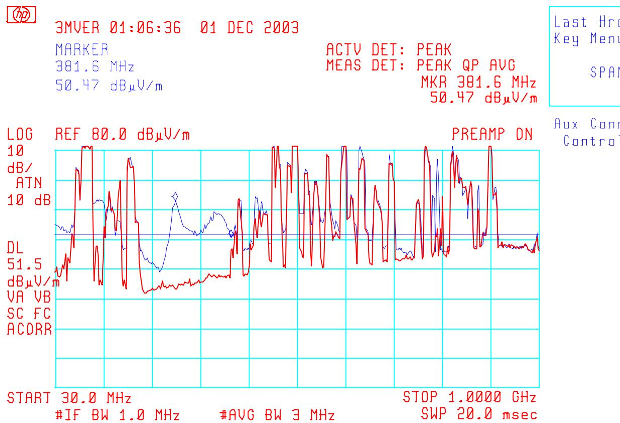
**Plot #2(a) - Lower 10 dB BW Point of the TLF with 100 MHz Antenna
