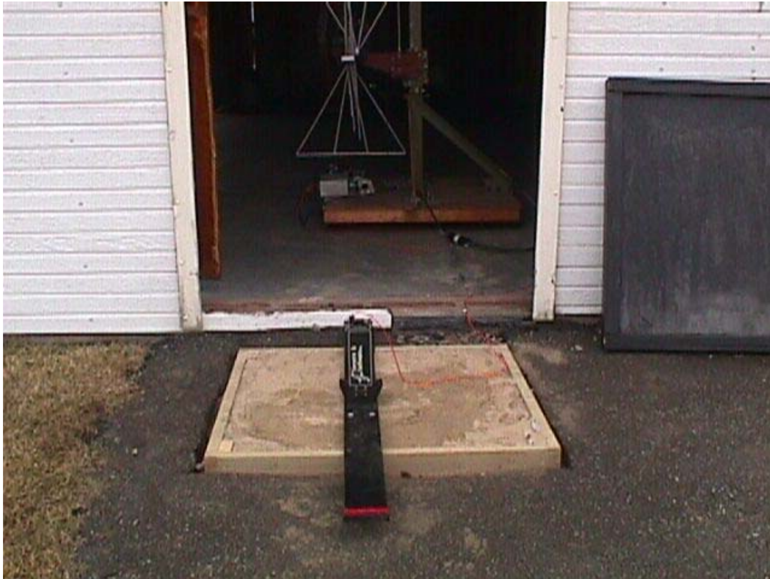
Test Configuration #3: Pulse Ekko 100 with 50 MHz Antenna
