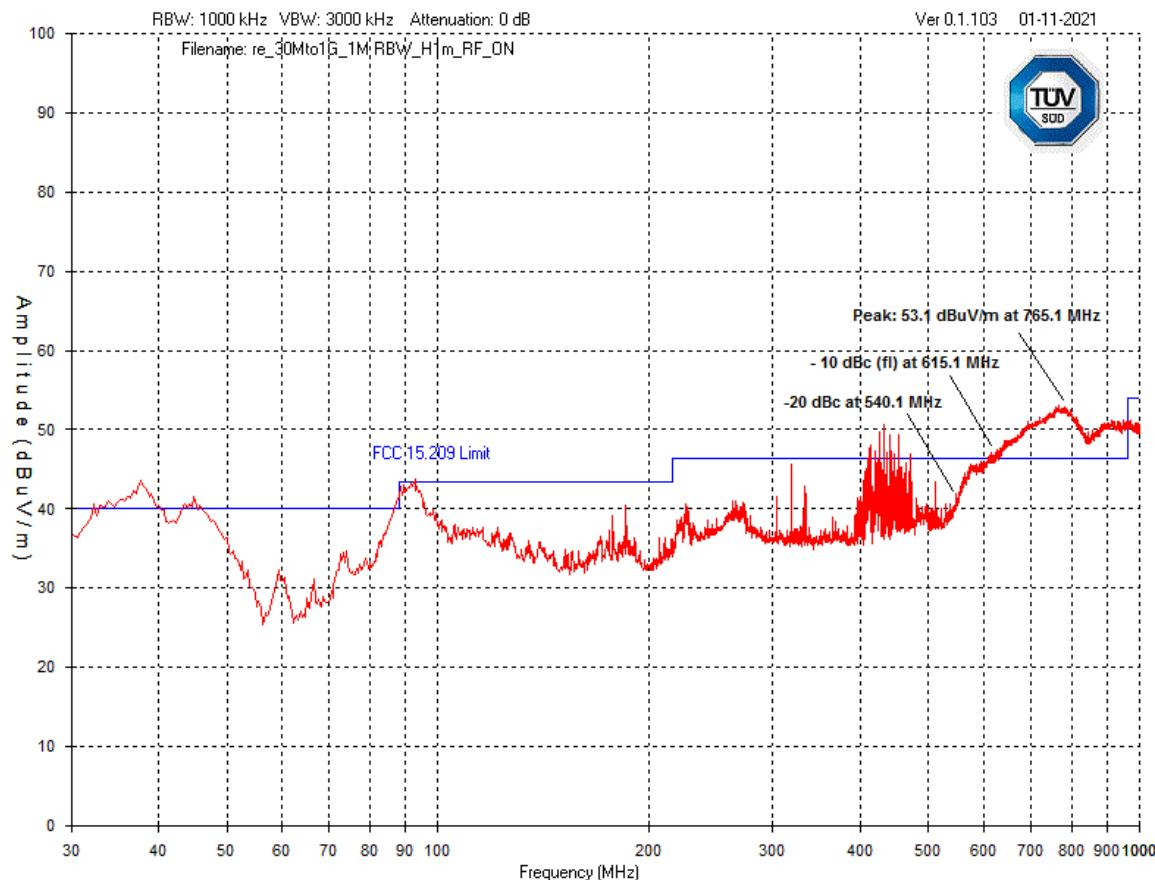
Note: Emissions shown as exceeding the 15.209 Quasi-peak limit as shown above, occurring below 500 MHz, were determined to be not part of the intentional UWB signal<sup>1</sup>. Those emissions are measured as part of the radiated unintentional digital emissions<sup>1</sup>, subject to the limits in 15.109 and/or 15.209 as documented later in this report.
