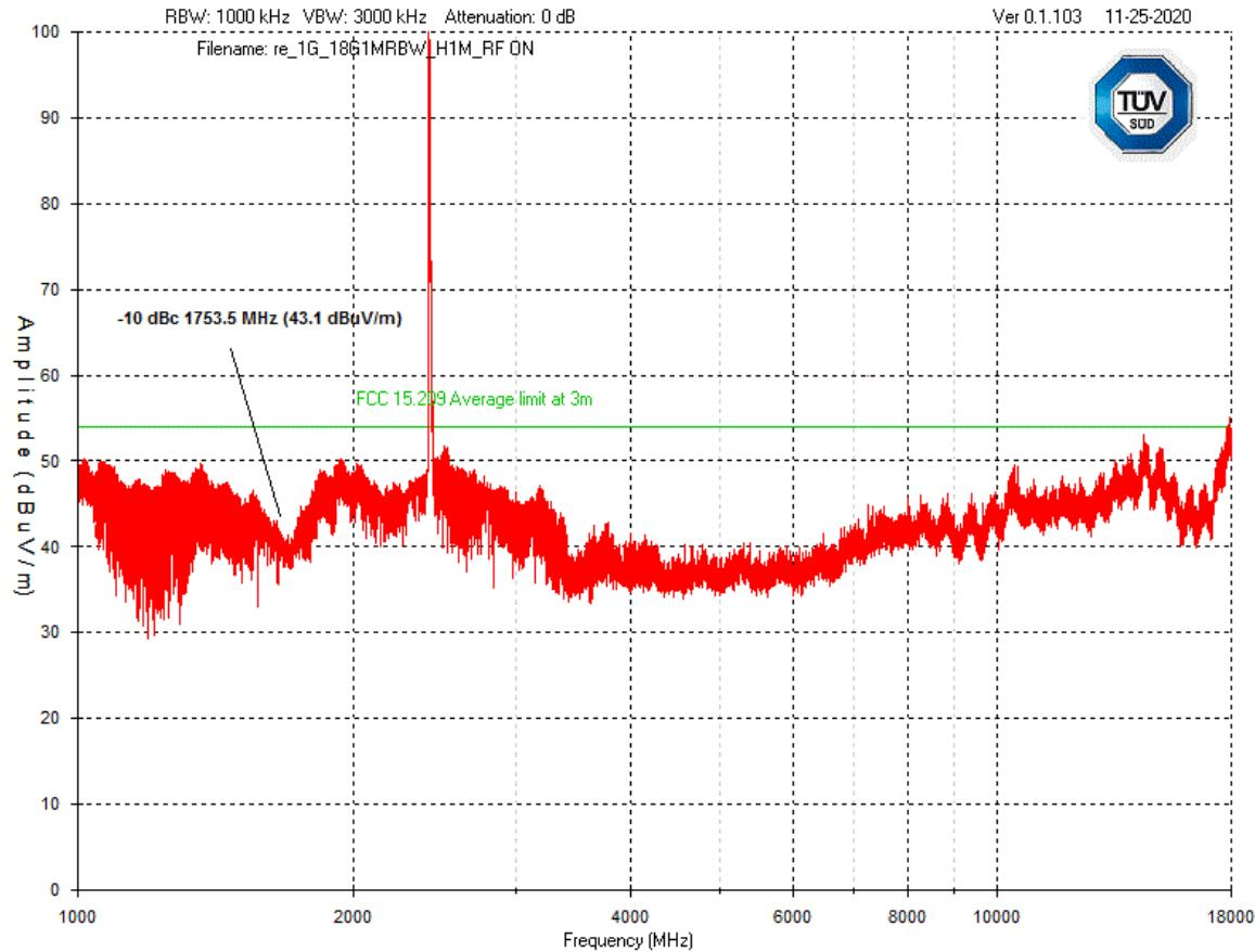
Note: The field strength drops below the 20 dB point from the peak (to 33.1 dBuV/m) at 3.751 GHz. The 20 dB point was measured using a 100 kHz resolution bandwidth.
