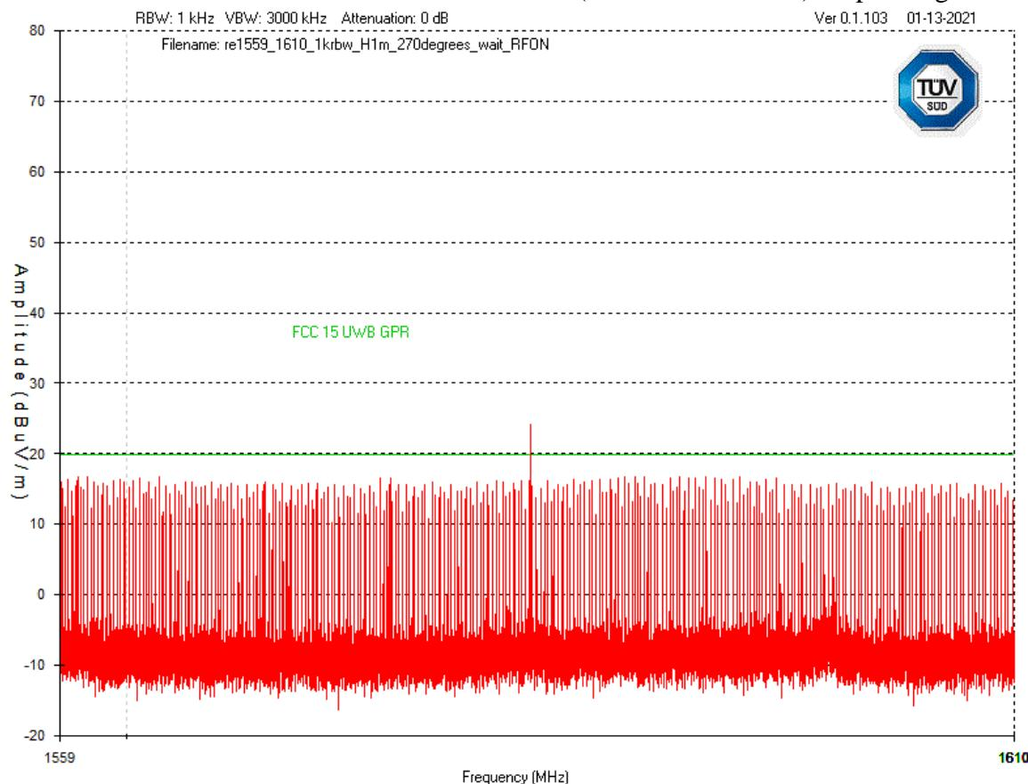
Note: The emission shown at 1584 MHz was determined to be an unintentional digital emission not related to the intentional UWB transmission.
