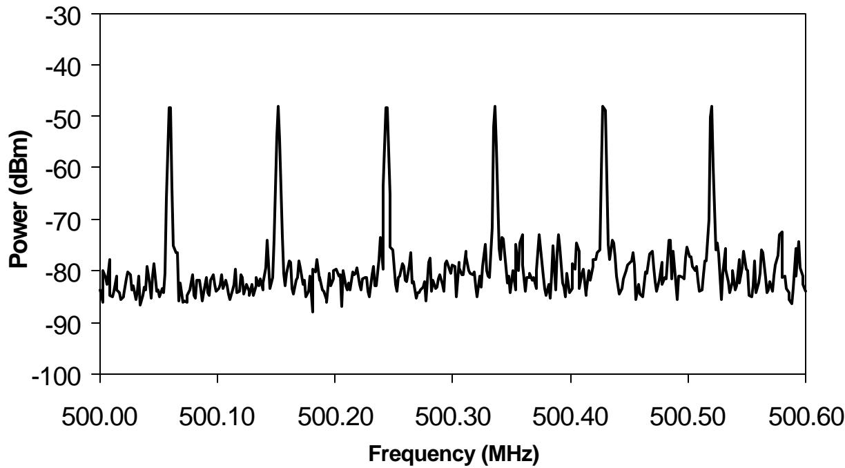
PRF measurements for Noggin 500 system. Measured PRF was 91.5 kHz.
