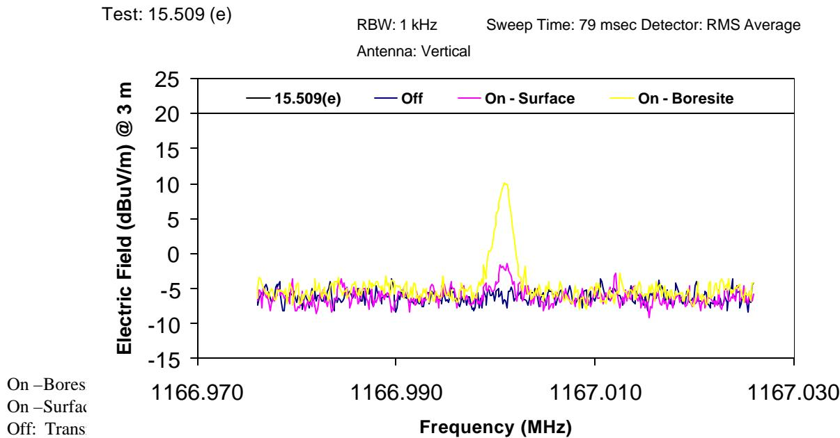
**Note:** The signal as displayed in yellow was measured when the EUT was lifted off the ground. This was done to detect the signal since it was too low when the EUT was laid on the ground.
