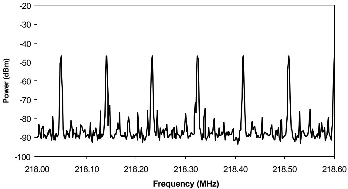
**6.3.5.2. Radiated Emissions with the EUT in Direct Contact with the Sand Soil Ground Plane**
