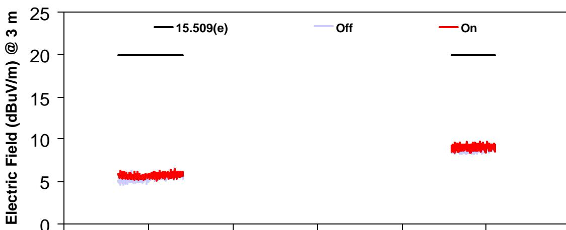
The spectrum produced by the GPR transmitter is a line spectrum. An example of the line spectrum produced by the transmitter in the GPS bands using sweep rate of 79 msec and a resolution bandwidth of 1 kHz is shown below. The electric field level was measured at 10 of these peaks in the frequencies specified in 15.509(e). These values are tabulated below. The transmitter was 0.6 m from the EMC antenna for the measurements but they have been corrected to a 3 m separation.
