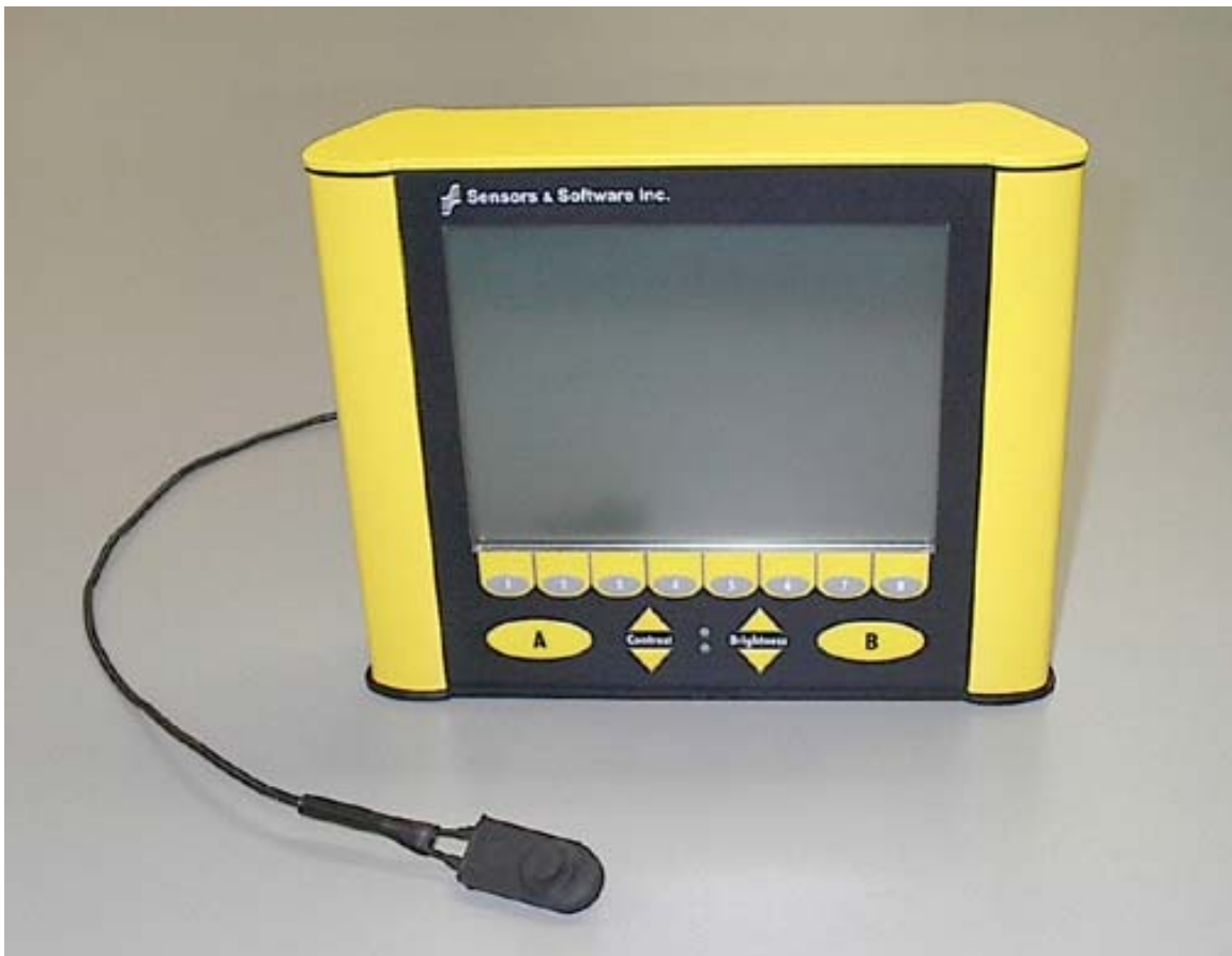
Switch used to control Noggin 1000 transmitter. This switch must be depressed for the Noggin transmitter to operate.
