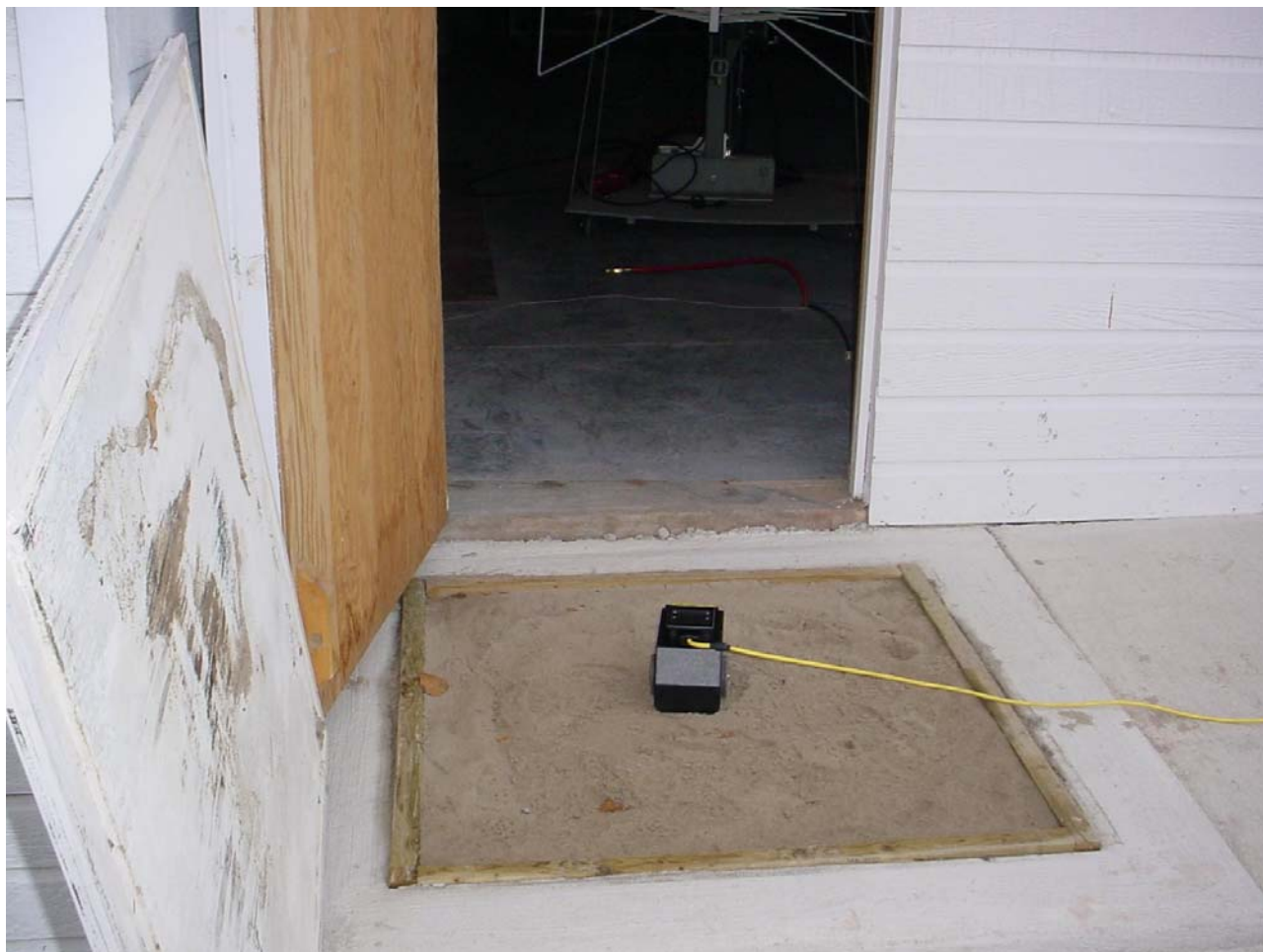
Plot #3: Radiated Emissions Test Setup
