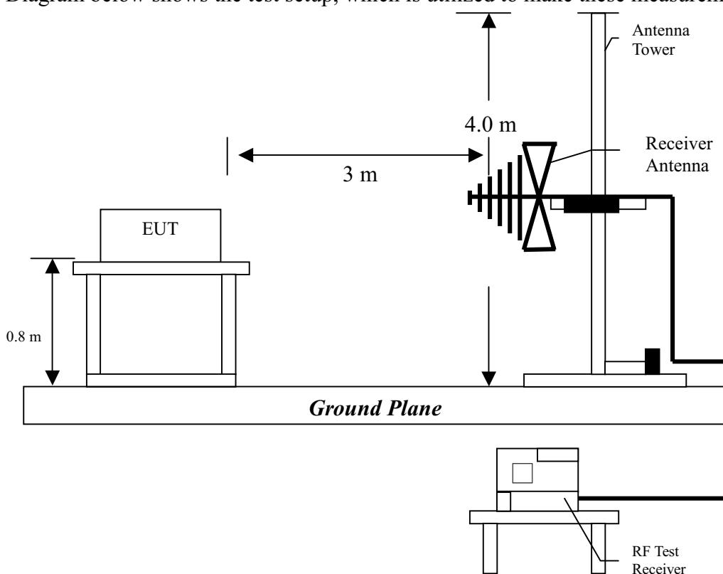
The signal is maximized through rotation and placement in the three orthogonal axes. Radiated emission measurements were performed from 30MHz to 25GHz. Spectrum Analyzer Resolution Bandwidth is 100kHz or greater for frequencies 30MHz to 1GHz, 1MHz – for frequencies above 1GHz.
