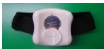
Remove the battery compartment cover from the bottom of the transmitter.
