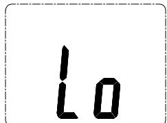
Lowest possible temperature setting reached. The unit does not function at temperatures below 25°C (77°F)
