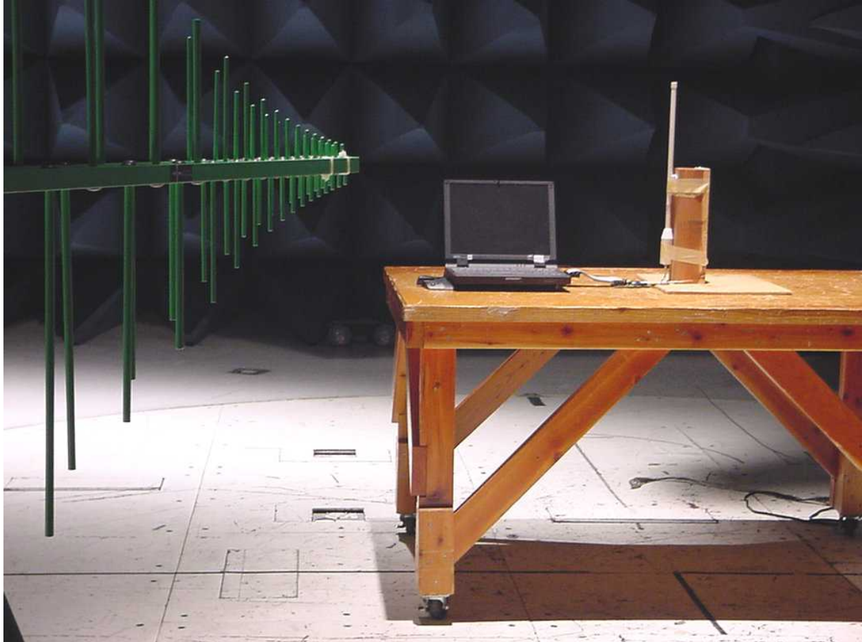
Photograph 2. Radiated Emission Limits (Below 1 GHz), Test Setup
