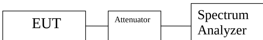
Figure 3. Power Output Test Setup
