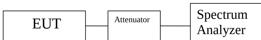
Figure 4. Power Spectral Density Test Setup
