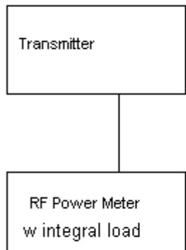
POWER OUTPUT: 1 Watt appears to meet the FCC requirements.
