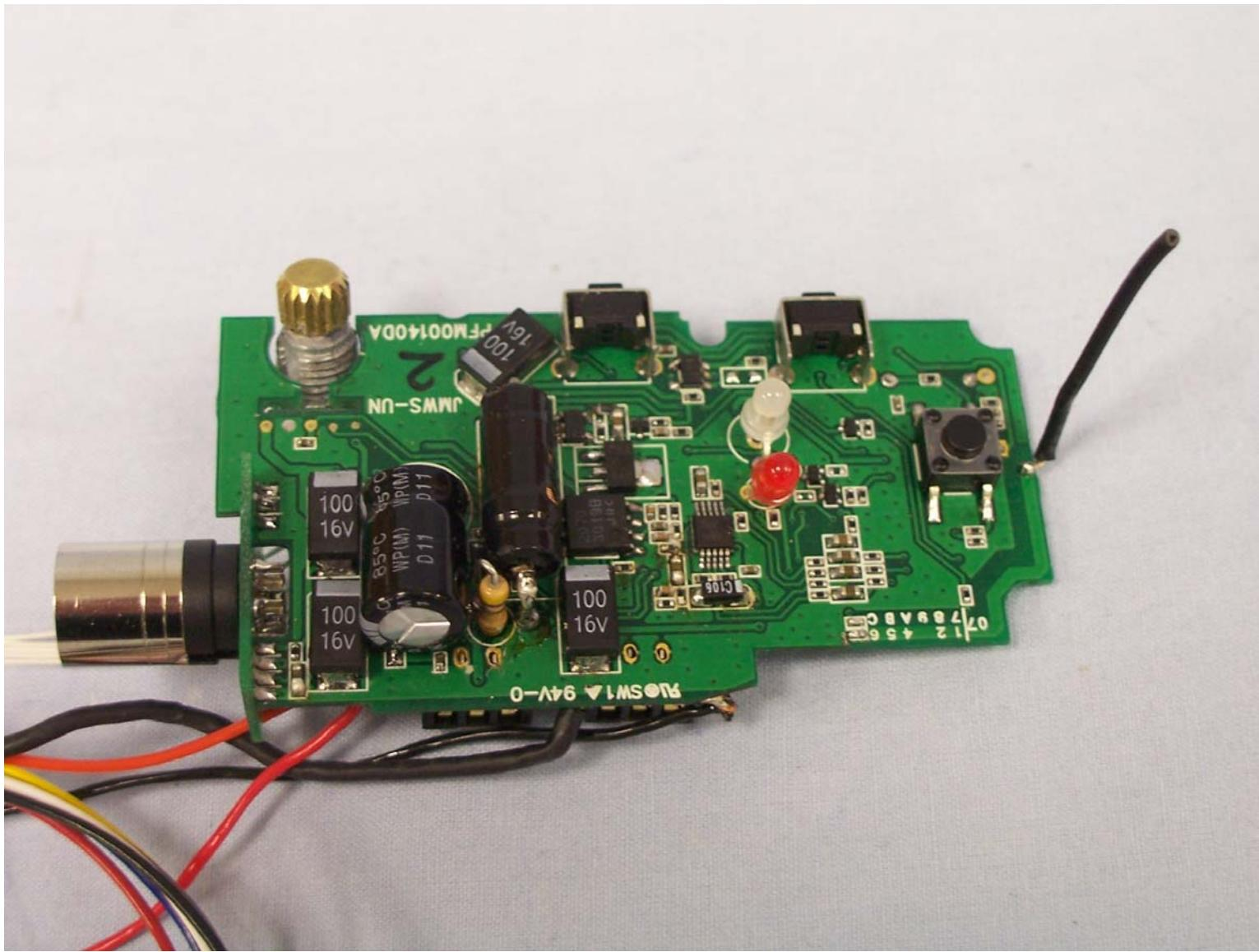
This is a jumper that was installed in place of a missing trace.
