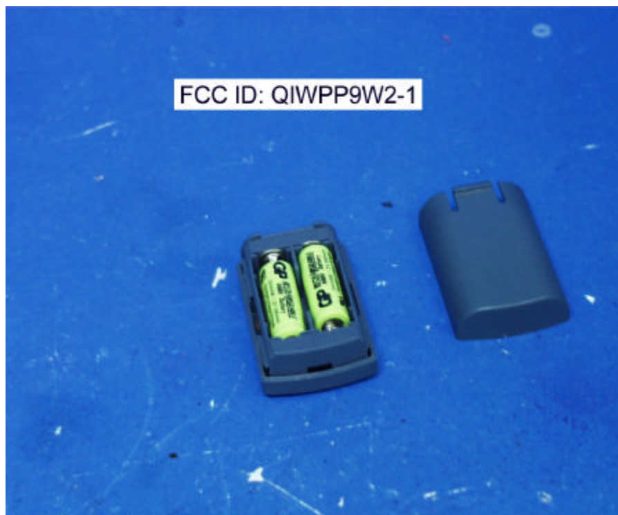
Battery Box Inner Photo 3
