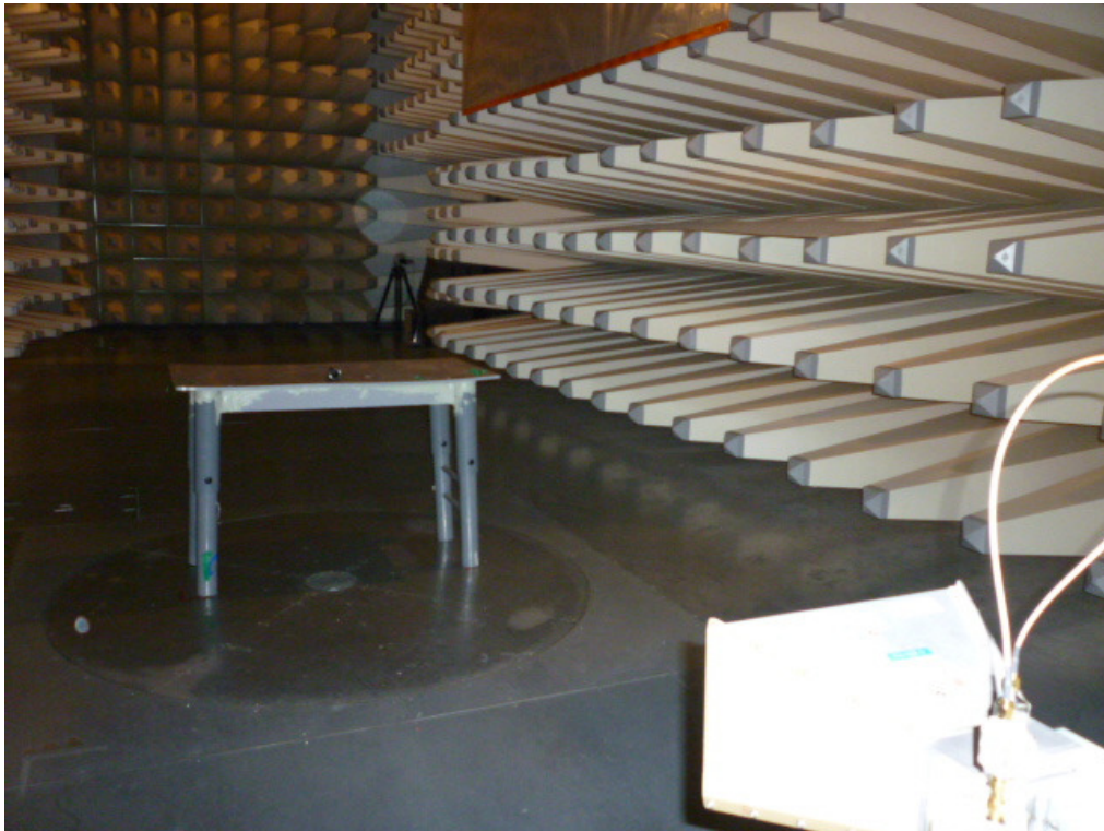
Set-up for Radiated Emission
