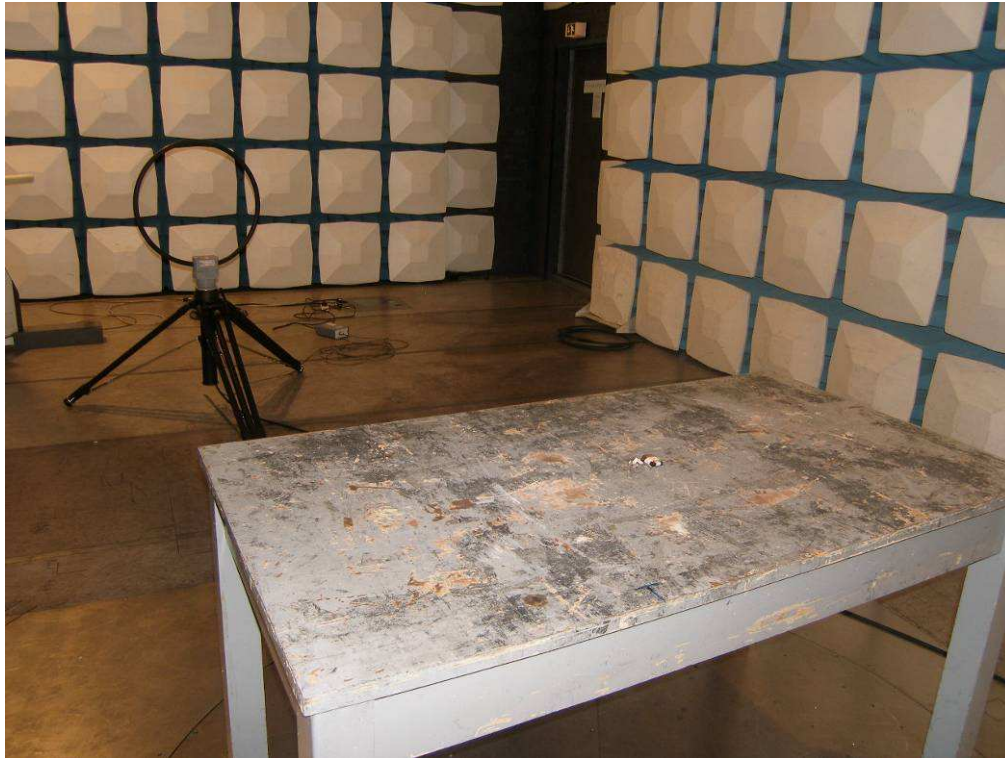
Photograph 2: Set-up for Spurious Emissions (30MHz-1GHz)
