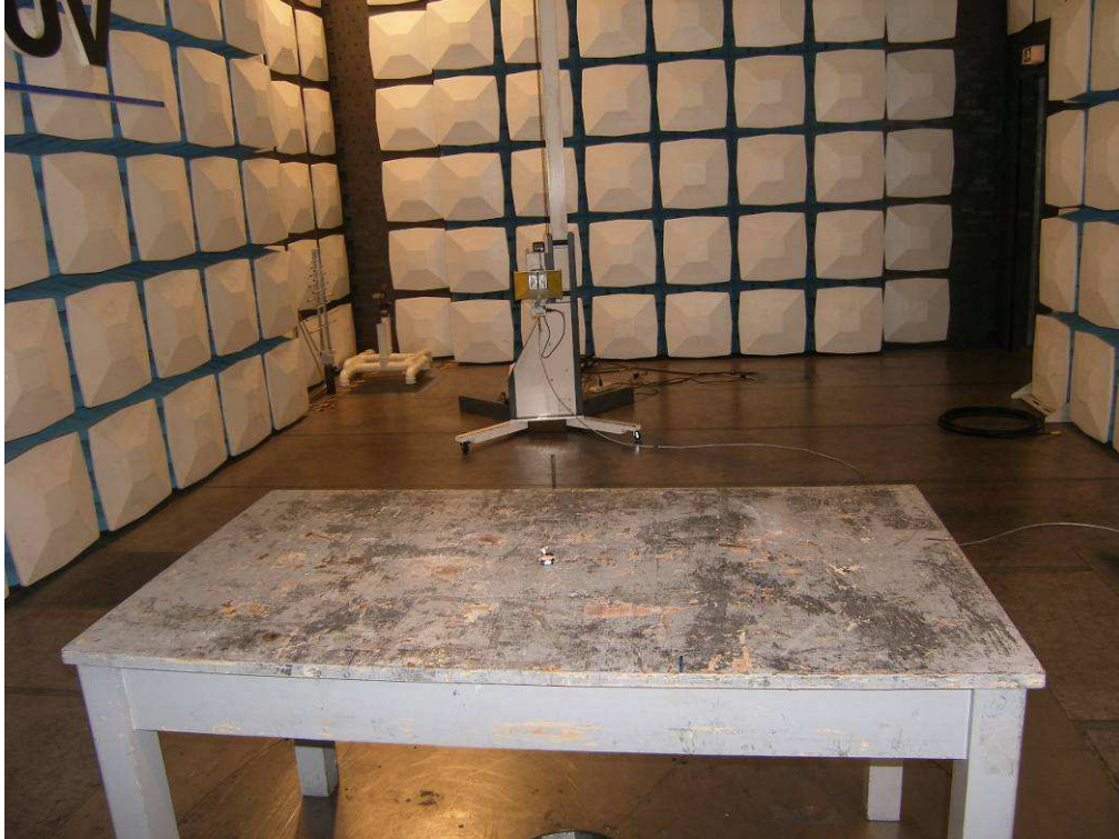
Photograph 4: Set-up for Spurious Emissions (18GHz-26GHz)
