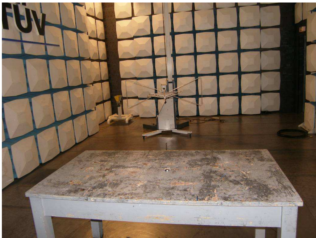
Photograph 2: Set-up for Spurious Emissions (30MHz-1GHz)
