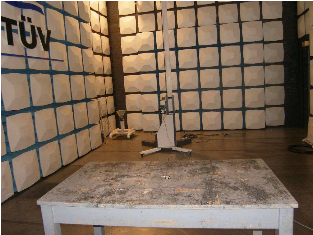
Photograph 4: Set-up for Spurious Emissions (18GHz-26GHz)
