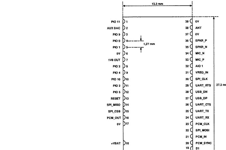
Note: Module thickness < 2.5 mm
