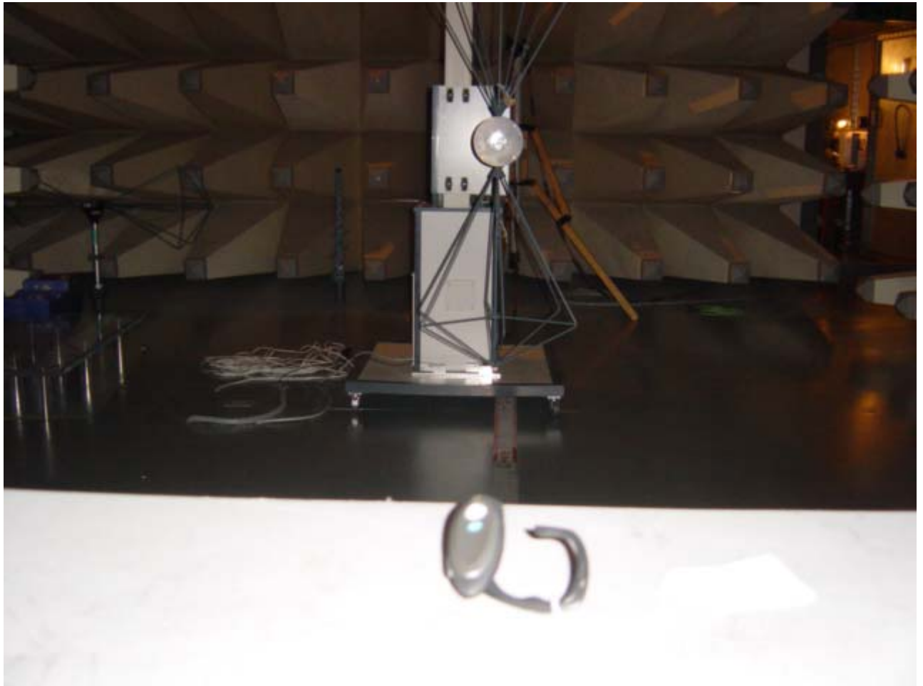
Set-up for Radiation Emission (Transceiver)
