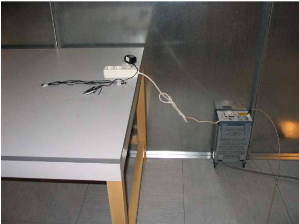
Set-up for Disturbance Voltage on AC mains
