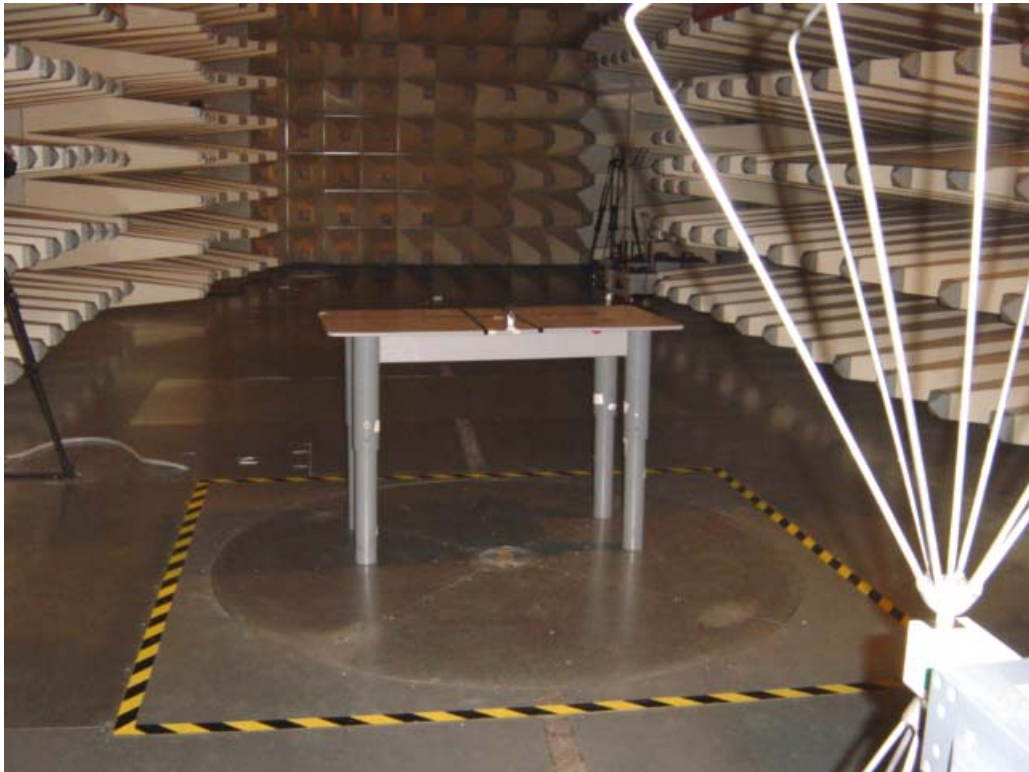
Set-up for Radiation Emission (Transceiver)
