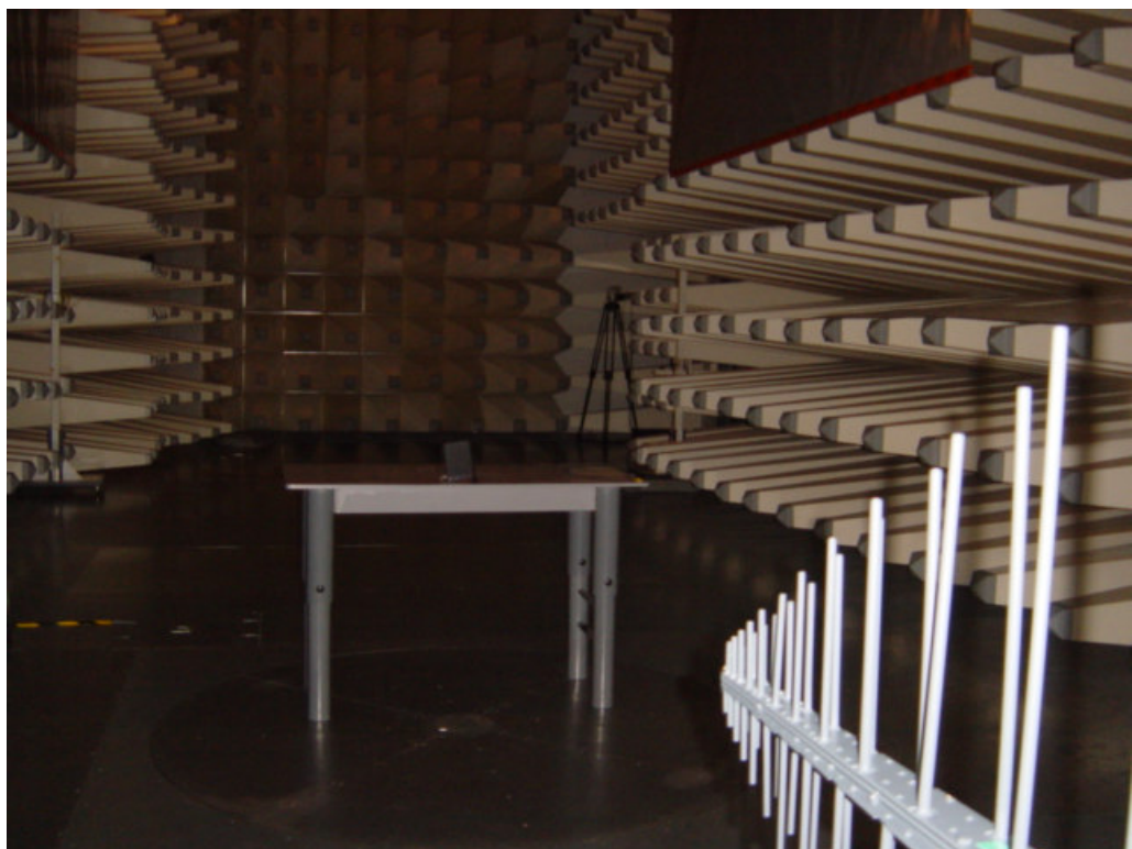
Set-up for Radiation Emission (Transceiver)
